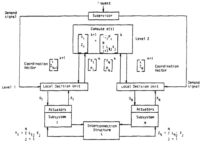
Fig. 2. Interaction prediction method hierarchical control.
