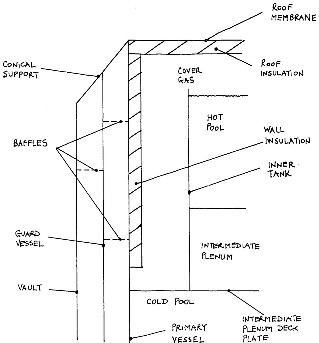
LAYOUT OF THE REACTOR UPPER STRUCTURE
