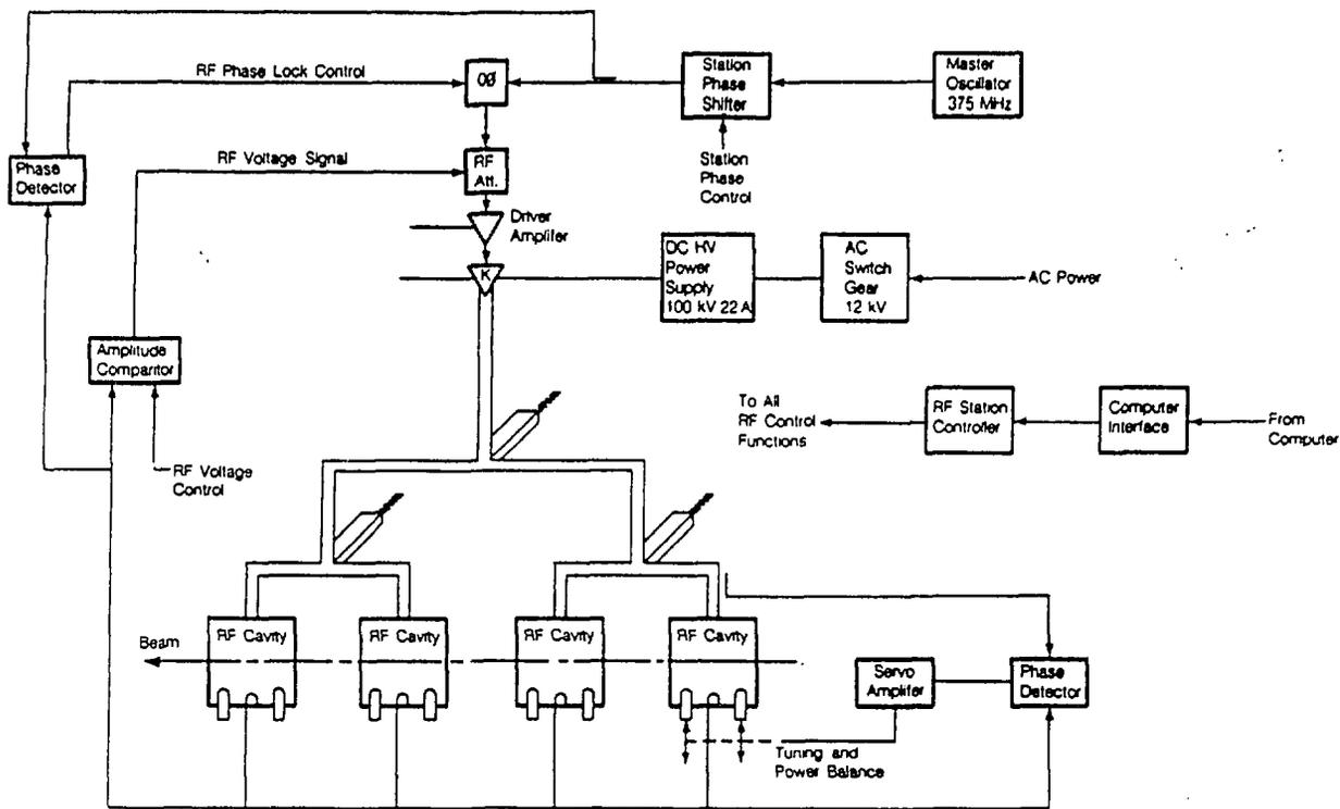
Master circuit diagram of rf system, indicating servo-loops to stabilize the amplitude and phase of the cavity fields.
