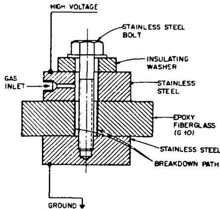
Fig. 4. Test specimen for VCL flange bolt
