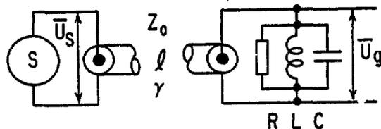
Fig. 2 Equivalent Circuit Diagram of Linac Cell
