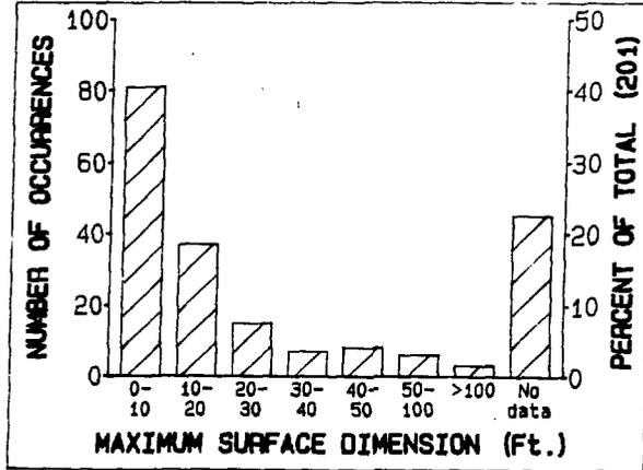
Figure 3. Maximum surface dimension size distribution for reported karst subsidence incidents.
