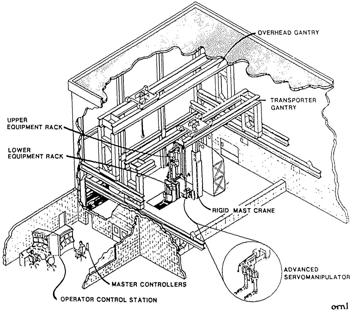
Fig. 1. The Advanced Integrated Maintenance System.
