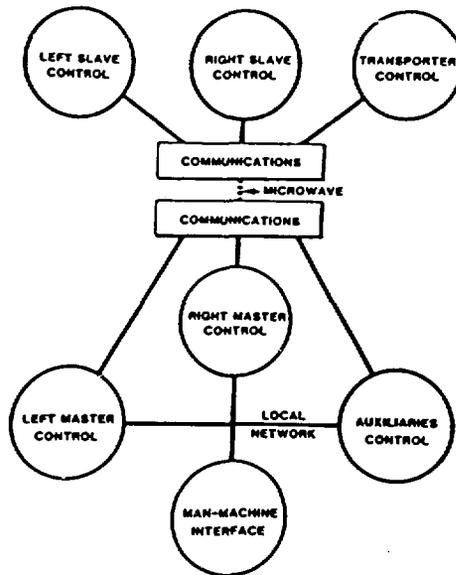
Fig. 2. AIMS control system block diagram.
