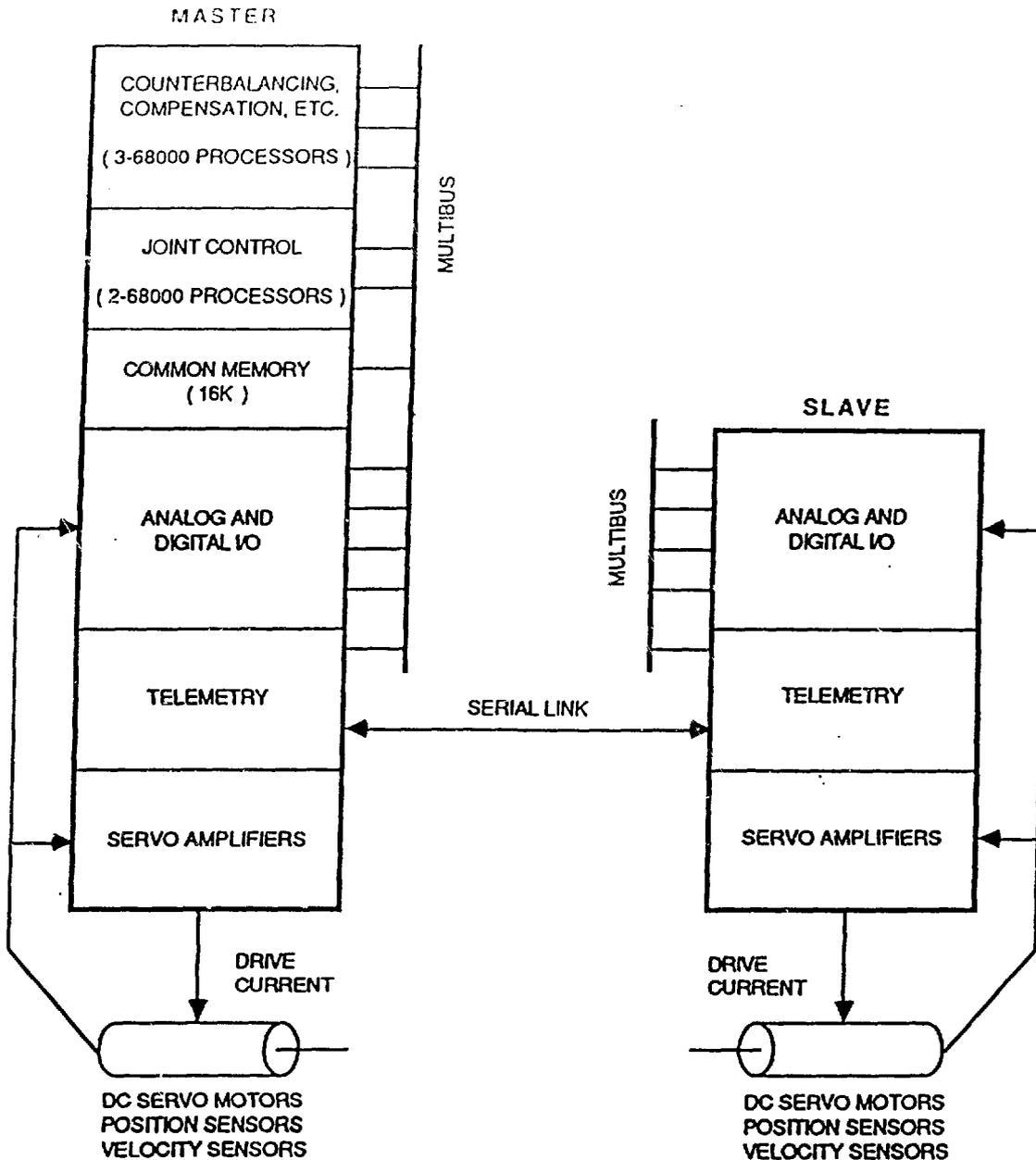
Fig. 8. Block diagram of the Advanced Servomanipulator (ASM) Controls.
