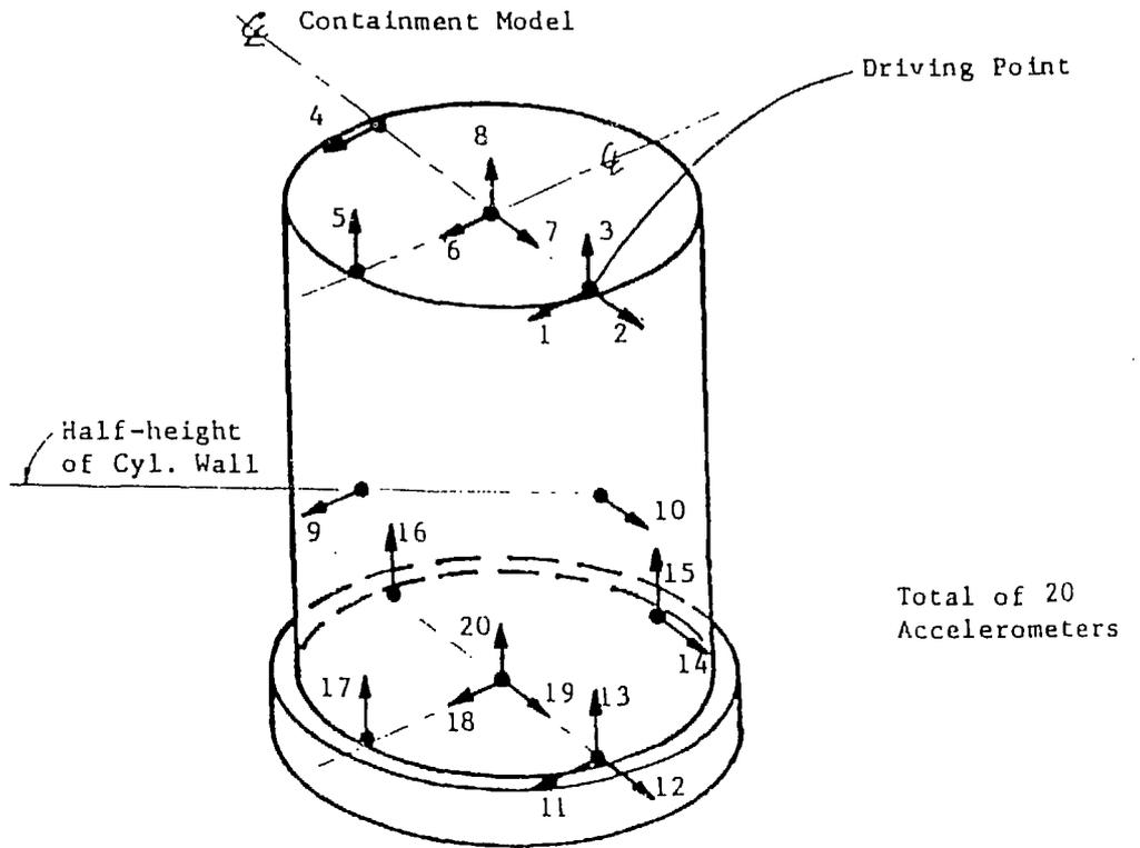
Figur 5. Vibration Test Instrumentation of Structure
