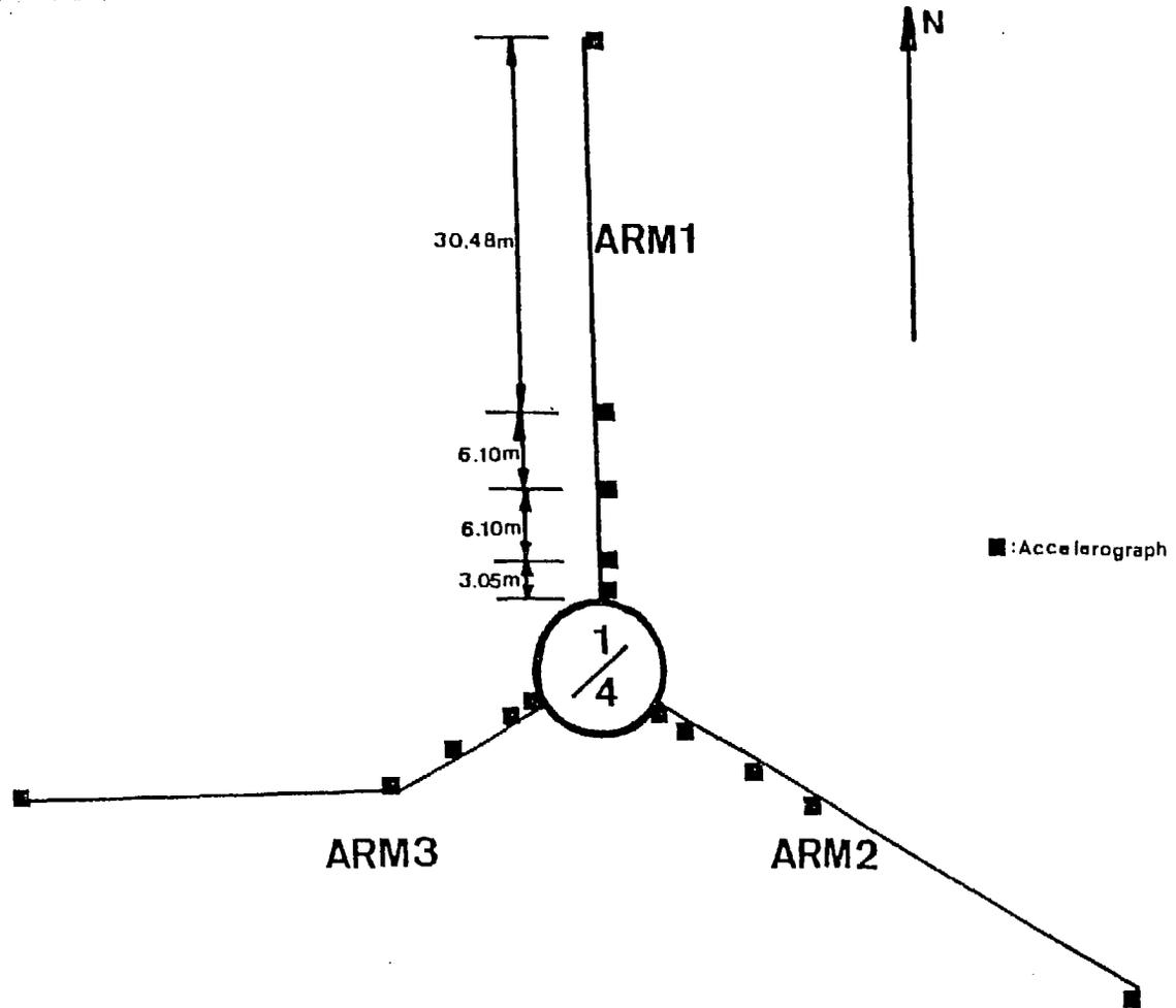
Figure 6. The Surface Instrumentation Array
