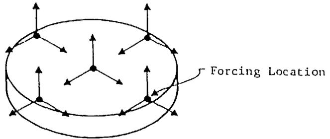
Figure 4. Vibration Test Instrumentation of Basemat
