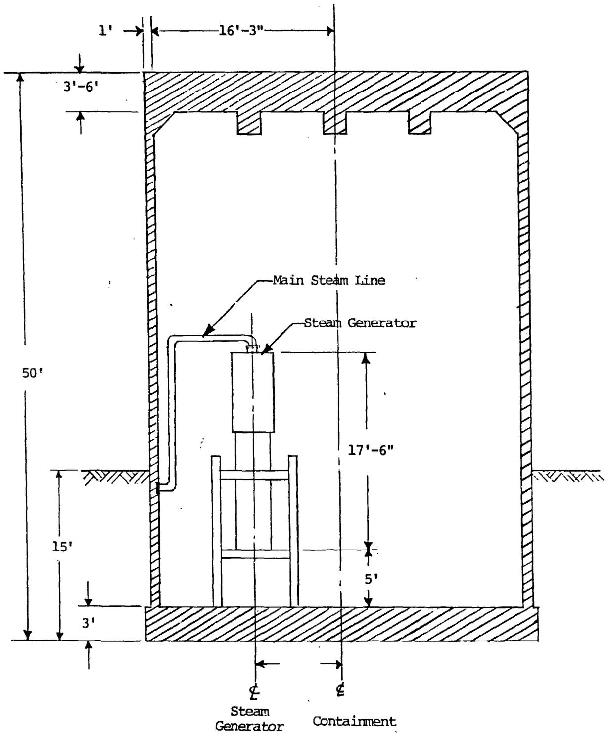
Figure 2. Cross Section of 1/4-scale Containment Model
