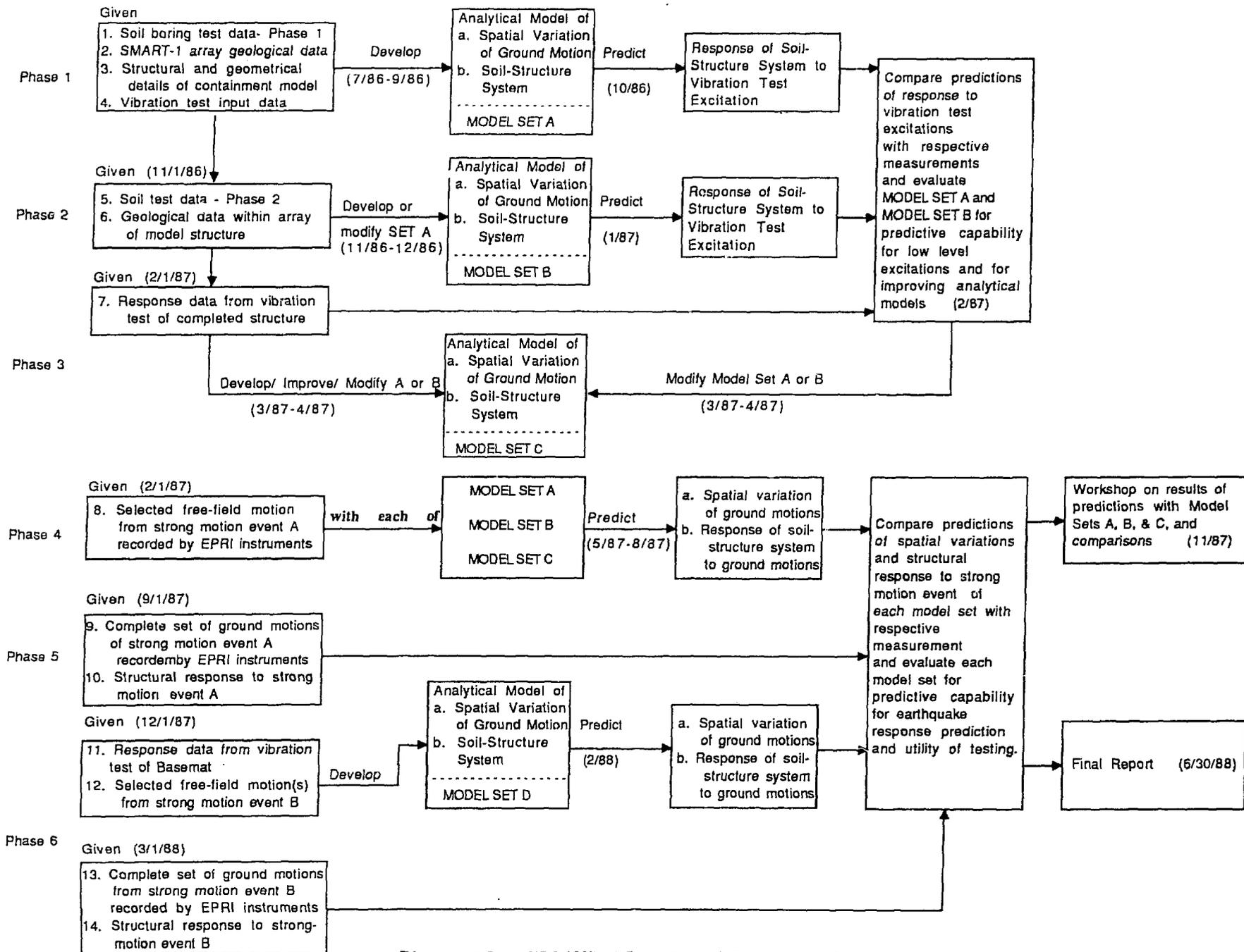
Figure 10. NRC/ANL Plan for Validation Program
