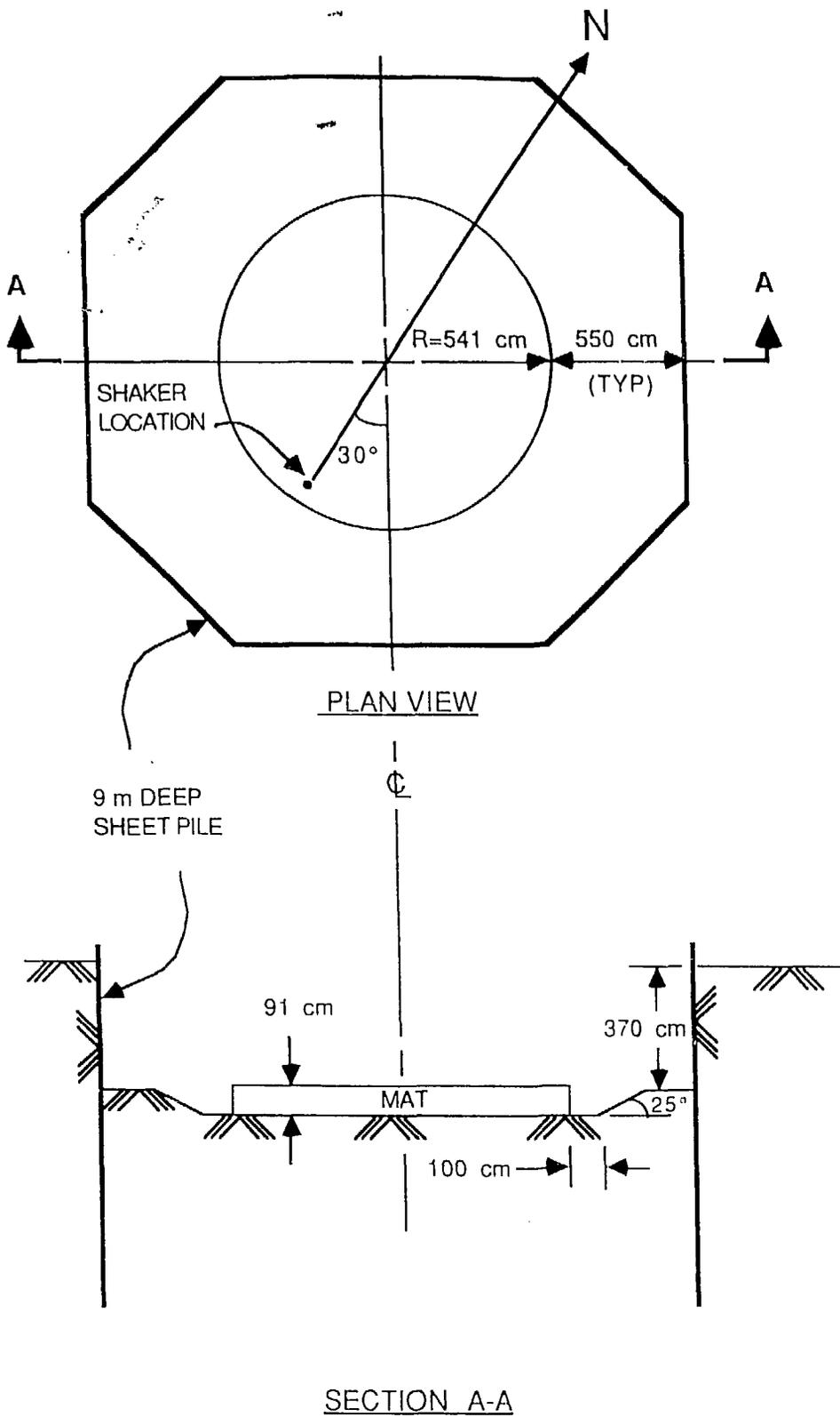
Figure 3. Configuration during Vibration Tests on Basemat
