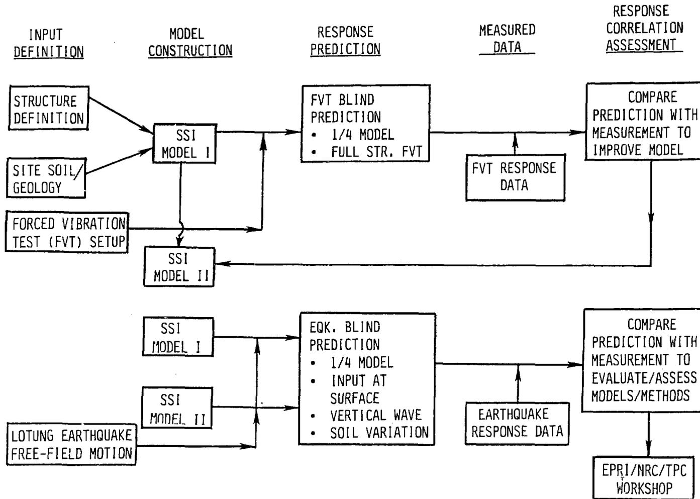
Figure 11. SSI Analysis for Lotung Seismic Experiment (EPRI Program)
