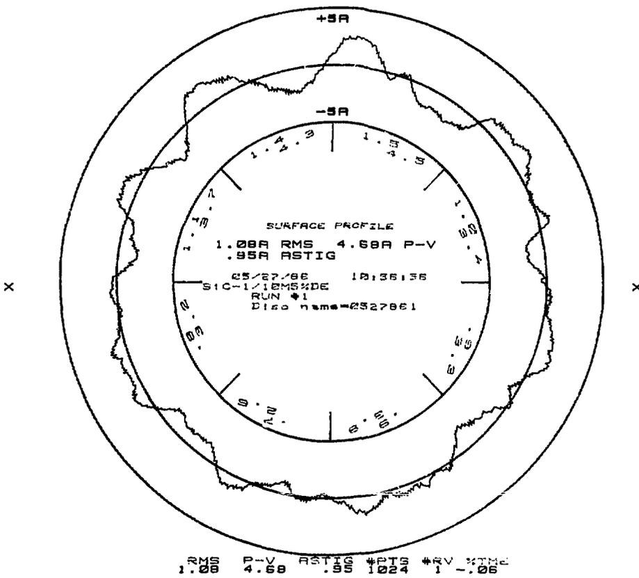
**FIGURE 7** Optical Hetrodyne Profilometer trace of a SiC surface after pitch polishing with 0.1 micrometer diamond: Test sample Number 2 of three.
