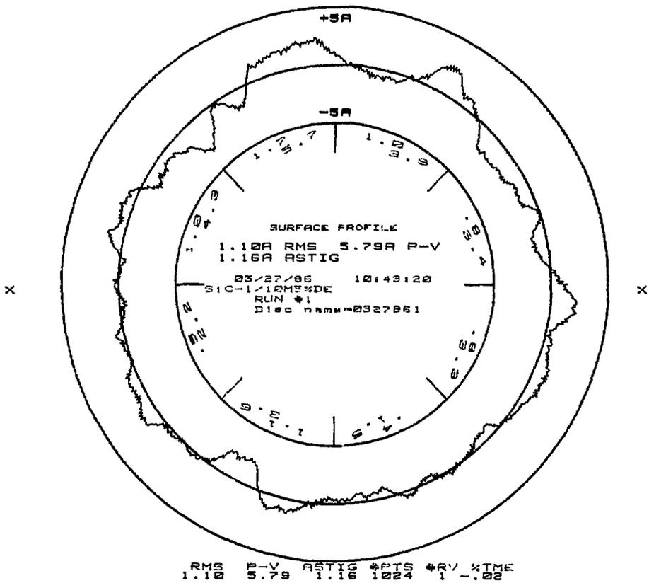
**FIGURE 8** Optical Hetrodyne Profilometer trace of a SiC surface after pitch polishing with 0.1 micrometer diamond: Test sample Number 3 of three.
