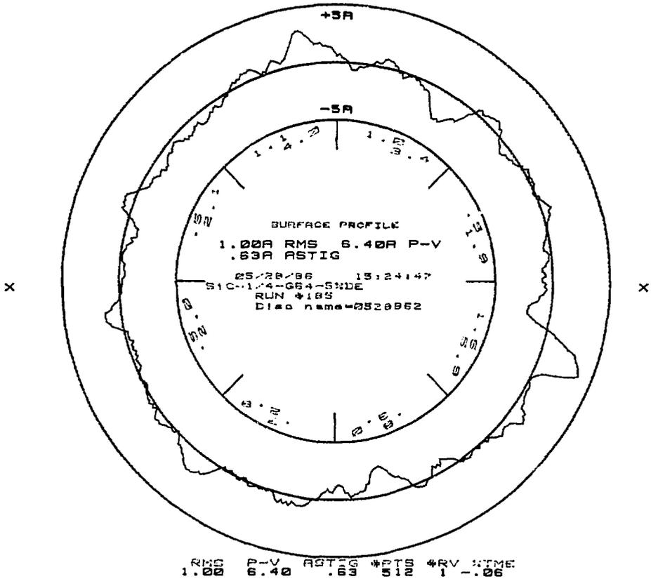
**FIGURE 6** Optical Hetrodyne Profilometer trace of a SiC surface after pitch polishing with 0.1 micrometer diamond: Test sample Number 1 of three.
