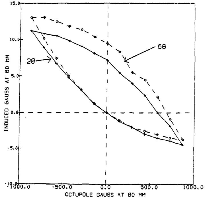
Figure 2. Magnetization produced in CBA main dipole coil by excitation of octupole trim coil. The units are gauss measured at the trim coil radius of 60 mm. The central dipole field was at the injection value of 0.4 T.
