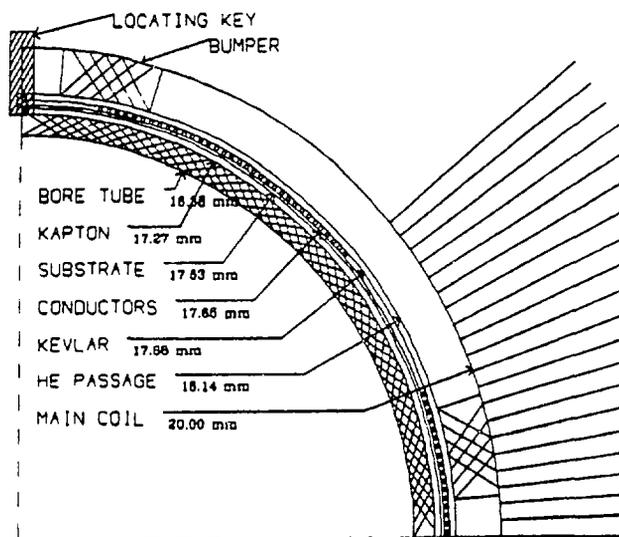
Figure 3. Cross section of SSC trim coil assembly.
