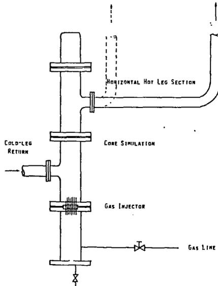
Fig. 4. Hot-leg Inlet with Horizontal Section Simulation Reactor Vessel Exit Geometry (short and long horizontal sections shown)
