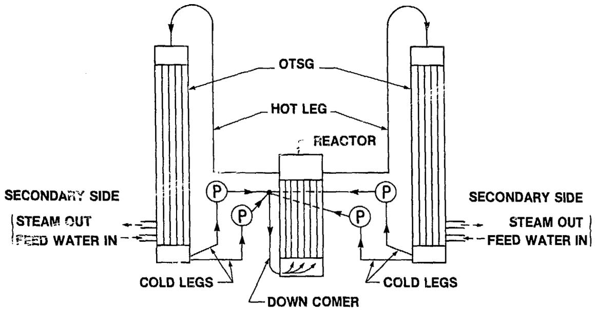
Fig. 1. Schematic of B&W 2x4 Loop Nuclear Reactor
