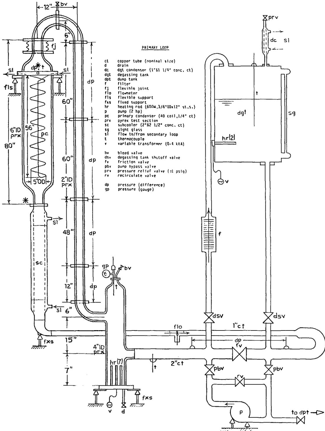
Fig. 5. Schematic of Freon 113 Boiling and Condensation Loop for Hot-leg U-bend Natural Circulation Study
