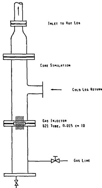
Fig. 3. Hot-leg Inlet of Vertically Straight Geometry without Horizontal Hot-leg Section
