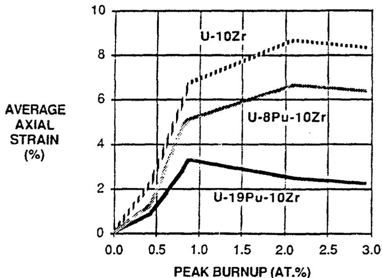
Figure 3. Burnup Dependence of Fuel Column Elongation for the 0, 8, and 19 wt % Pu Alloys.
