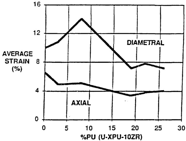
Figure 2. Plutonium Dependence of Fuel Deformation at 0.89 at.% Peak Burnup.
