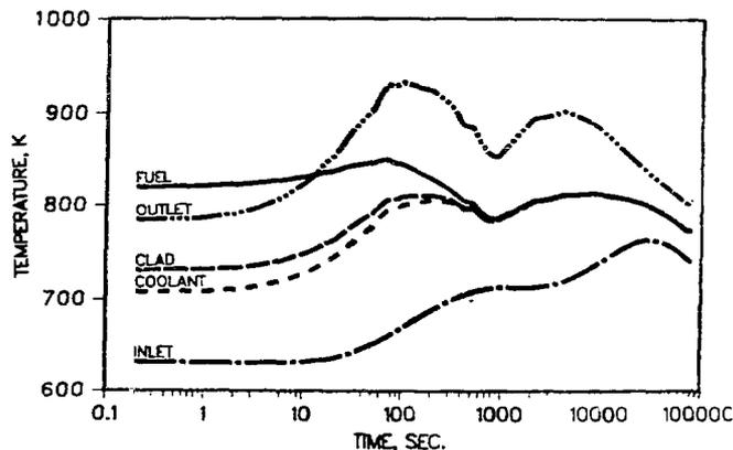
FIG. 1 IFR RESPONSE IN UNPROTECTED LOSS-OF-FLOW ACCIDENT
