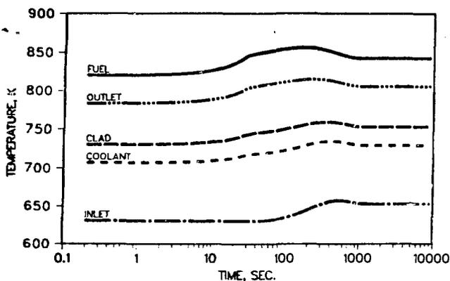
FIG. 2 IFR RESPONSE IN UNPROTECTED TRANSIENT OVERPOWER ACCIDENT
