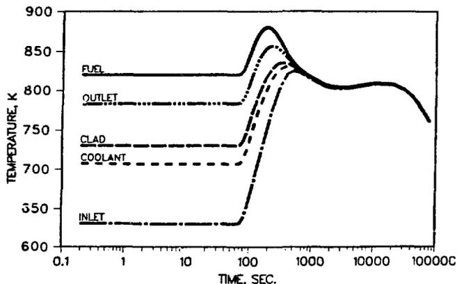
FIG. 3 IFR RESPONSE IN UNPROTECTED LOSS-OF-HEAT SINK ACCIDENT
