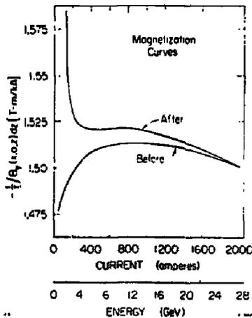
Fig. 8. Field integrals measured before and after subjecting a virgin PEP bending magnet to a magnetization cycle. Every PEP magnet was measured in this way with data taken from 1-27 GeV.
