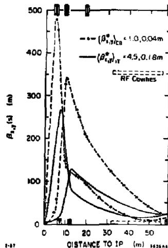
Fig. 6: Beta functions for the new colliding beam configuration of Table III around the Interaction Region (IR) and RF cavities.
