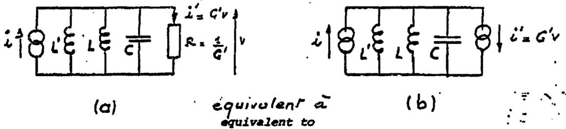
Fig. 11. Damping the oscillating circuit with a resistance or an equivalent current generator.
