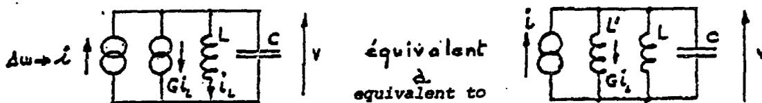
Fig. 9. Electrical equivalents of the servo of Fig. 7.
