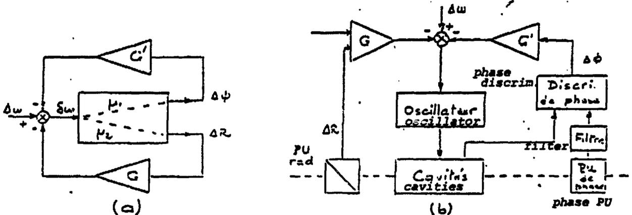
Fig. 12. Damping the system by means of an auxiliary loop.
