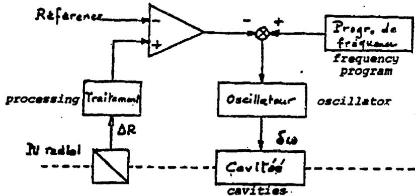
Fig. 2. First attempt at correcting the frequency program.
