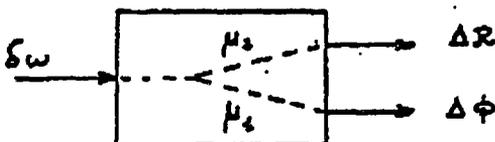
Fig. 3. Beam represented by equivalent black box.
