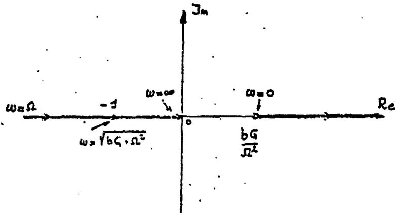
Fig. 8. Nyquist diagram for servo mechanism of Fig. 7.
