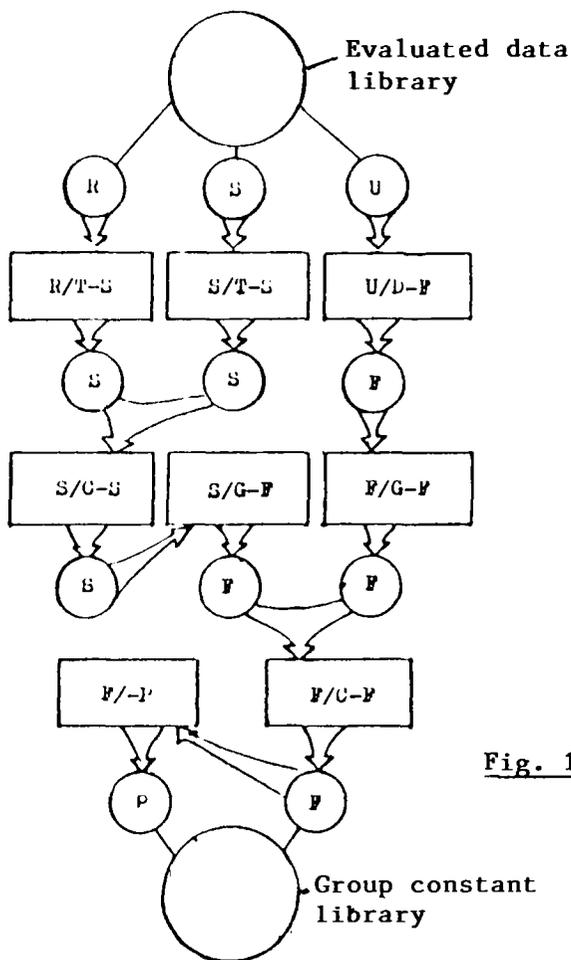
Fig. 1. System for converting evaluated neutron cross-section data into group constants
