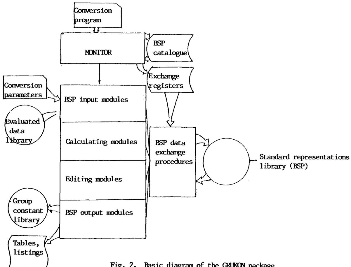
Fig. 2. Basic diagram of the GRUKON package
