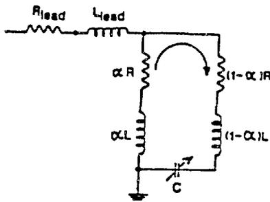
Fig. 2. Equivalent circuit of the compact loop antenna.
