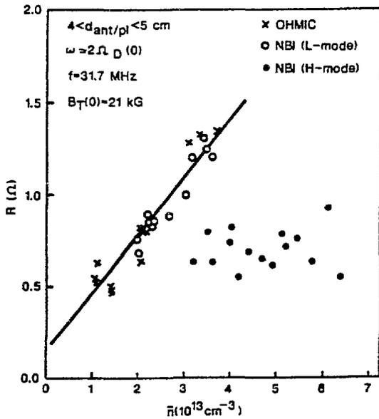
Fig. 4. Antenna loading vs. line-average density.
