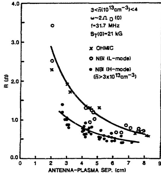
Fig. 5. Antenna loading as a function of the distance between the antenna Faraday shield and the plasma separatrix.
