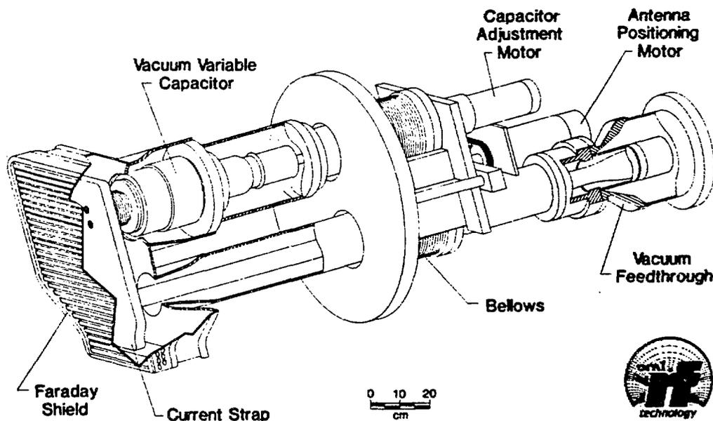
Fig. 1. Diagram of the compact loop antenna.
