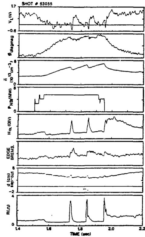
Fig. 3. Traces from a divertor discharge in DIII-D in which an H-mode transition is observed at  $t = 1575$  ms.
