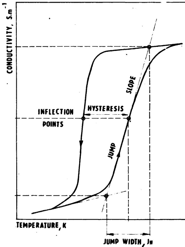
Fig. 11. Schematic view of the electrical conductivity jumps at melting and solidification (heating and cooling curves are marked by the arrows).
