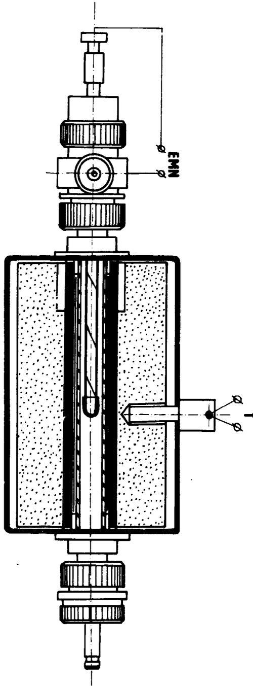
Fig. 8. The scheme of gas oxygen meter microfurnace
