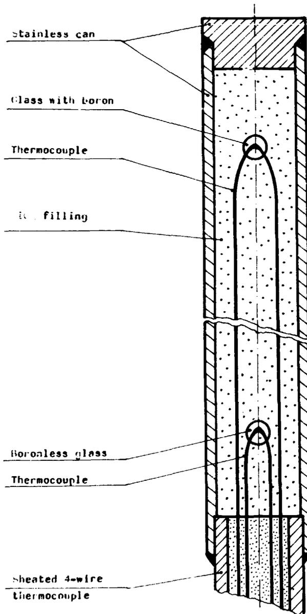
Fig. 13. Sectional view of the neutron flux meter
