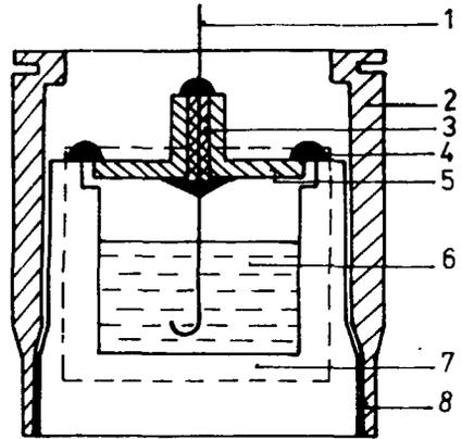
Fig. 3a. Design of the galvanic cell with brazed doped-thoria crucible
