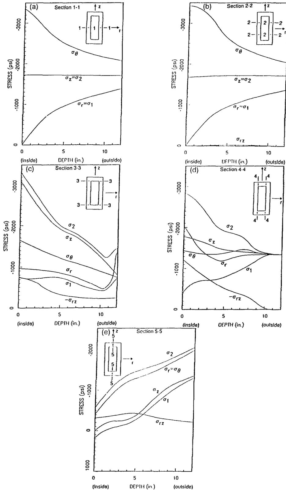
Figure 3. Stress plots at various sections.
