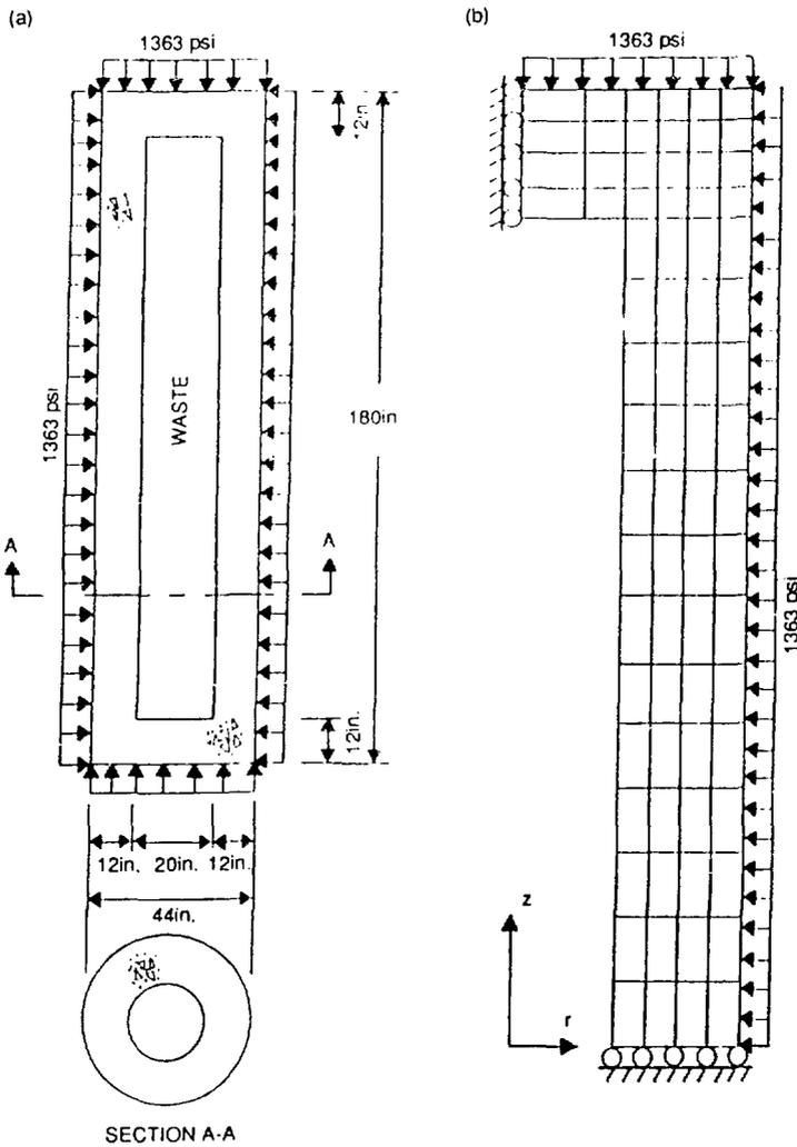
Figure 1. Container geometry and finite element mesh.
