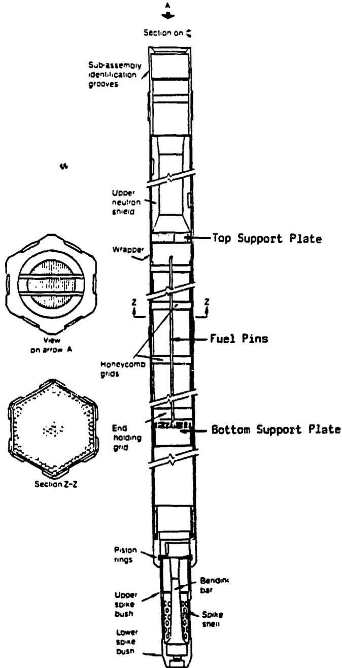
**FIG. 4** THE REFERENCE DESIGN FOR SUB-ASSEMBLY
