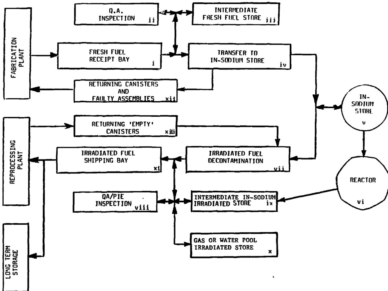
FIG. 3 SCHEMATIC OF FBR FUEL HANDLING ROUTE
