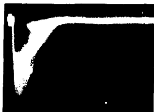
Fig. 6. The photography of the signals ( U = 3.3 kV; 400 A/div.; 50 ns/div.); H_{\perp} - component of the magnetic field which perpendicular to anode wires; H_{\parallel} - parallel component. a) H = 0 b) H_{\perp} = 12.2 kG, H_{\parallel} = 0 c) H_{\perp} = 9.1 kG, H_{\parallel} = 8.1 kG.
