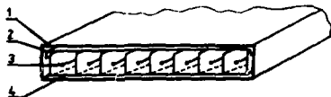
Fig. 1. The schematic view of plastic streamer tube: 1 - envelop; 2 - cover; 3 - anode wire; 4 - profile.
