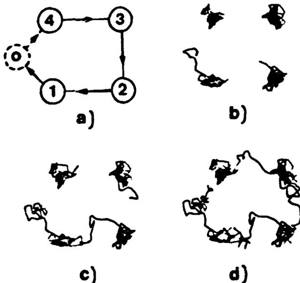
Fig. 2 : Example of  $\text{F}^-$  cyclic jumps in  $\text{CaF}_2$ . Trajectories of  $\text{F}^-$  ions at different timesteps ( $\Delta t = 0.5 \cdot 10^{-14} \text{s}$ ): a) schema, b)  $40 \Delta t$ , c)  $120 \Delta t$ , d)  $250 \Delta t$ .
