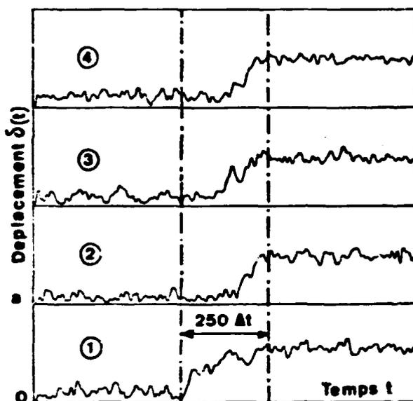
Fig. 3 : Diagram representing relative displacements of  $F^-$  ions from their initial position during the sequence of Fig. 2. The jump distance is given by  $a/2$ .
