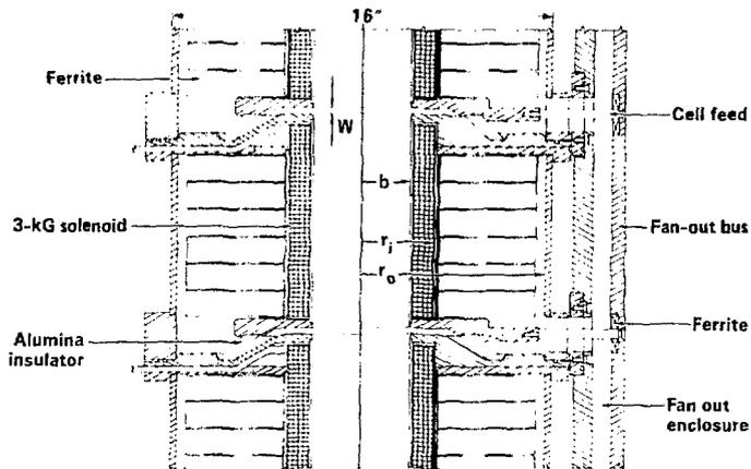
Figure 2. Cross-section of a typical low-gamma 10-cell module of the new 150-kV accelerator cell.
