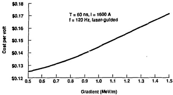
Figure 5. Driver cost vs gradient.
