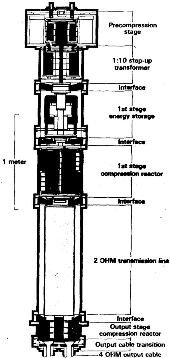
Figure 3. Cutaway view of MAG-1D.
