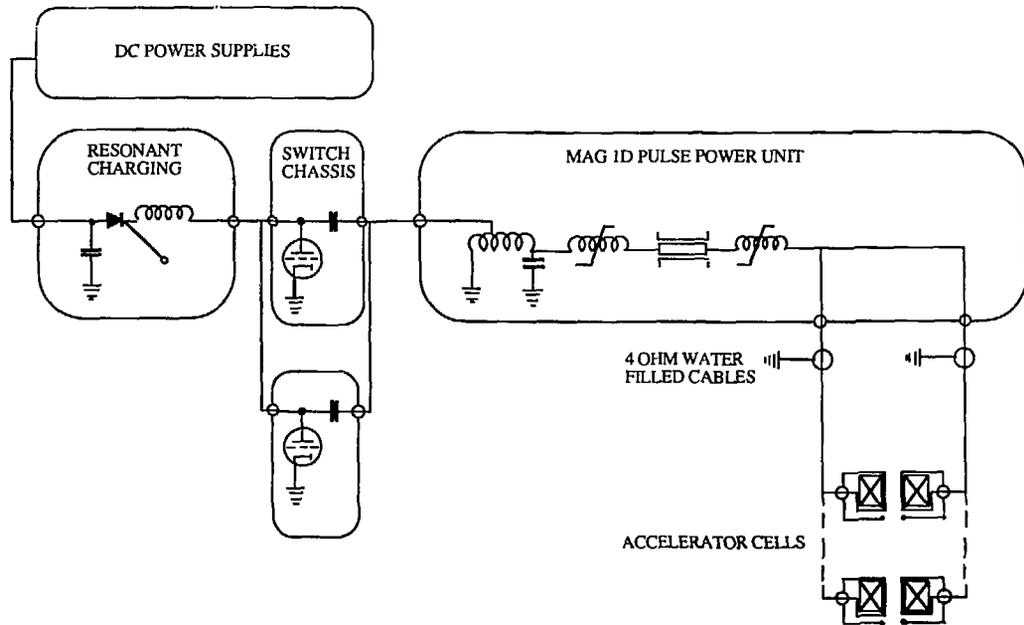
Figure 1. Schematic of baseline design of induction linac.
