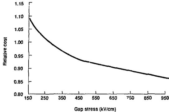
Figure 7. Relative costs vs gap stress.
