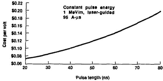
Figure 4. Induction driver cost vs pulse length.
