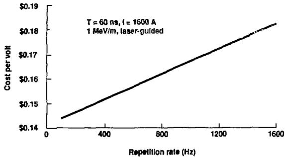
Figure 6. Driver cost vs repetition frequency.
