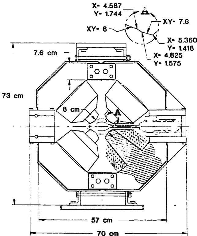
Fig. 2. End View of Quadrupoles
