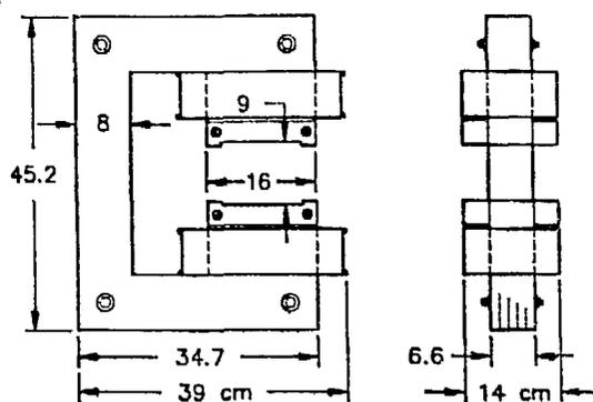
Fig. 4. Vertical Correction Magnet
