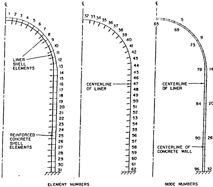
Figure 2. Discretization of Containment Model
