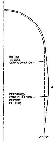
Figure 3. Vessel Deformation at Impending Failure
