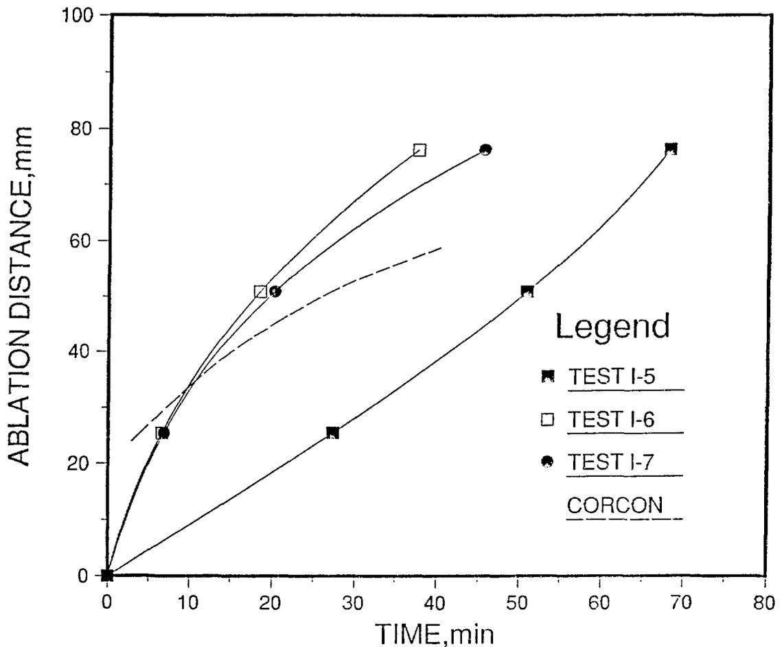
Figure 5. Ablation Distance vs. Time during HCCI Tests.
