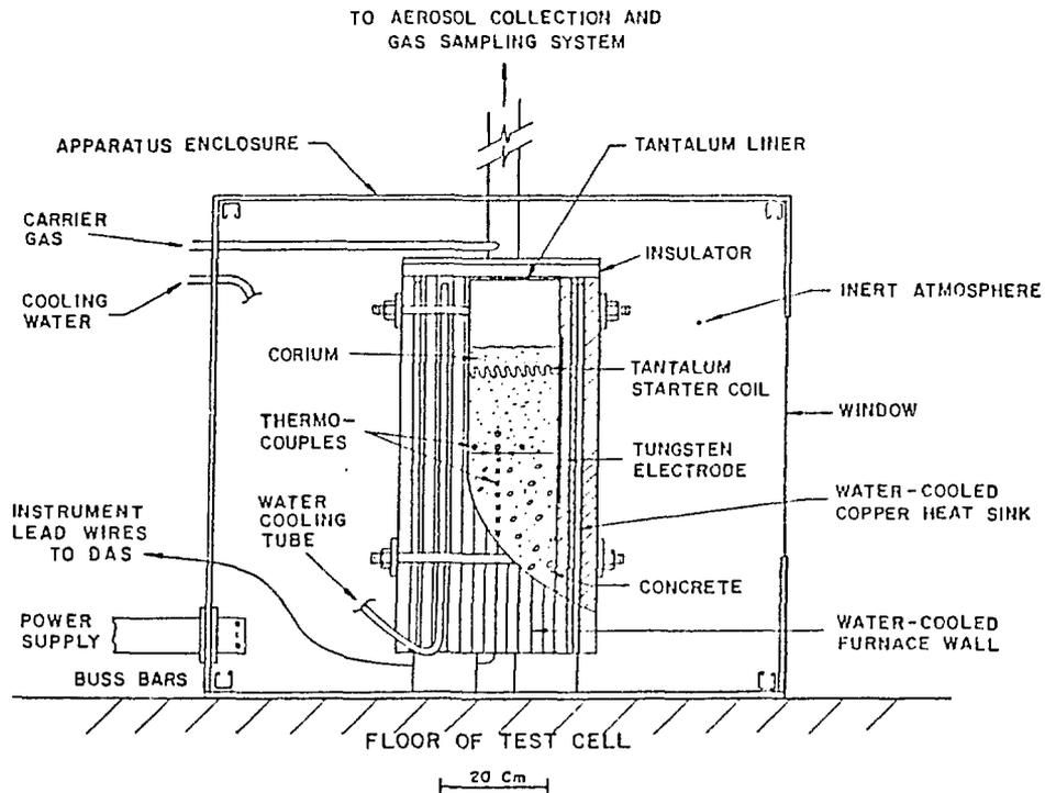
Figure 1. Illustration of Apparatus for Intermediate-Scale MCCI Tests.
