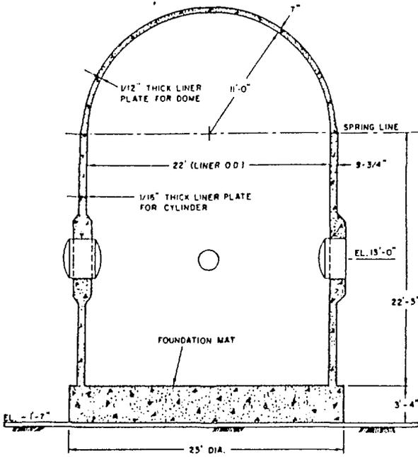
Figure 1. Reinforced Concrete Containment
