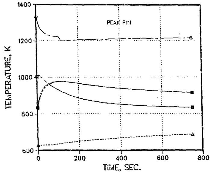
Figure 1. Illustration of Inherent Response of Innovative Liquid Metal Reactor to Unprotected Loss-of-Flow Event.
