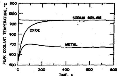
Fig. 4. Loss-of-Flow Without Scram for Large Reactors (1350 MWe).
