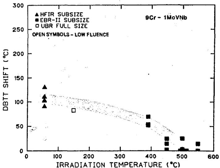
Fig. 1. Increase in DBTT as a function of irradiation temperature for (a) 12Cr-1MoVW and (b) 9Cr-1MoVNb steel.
