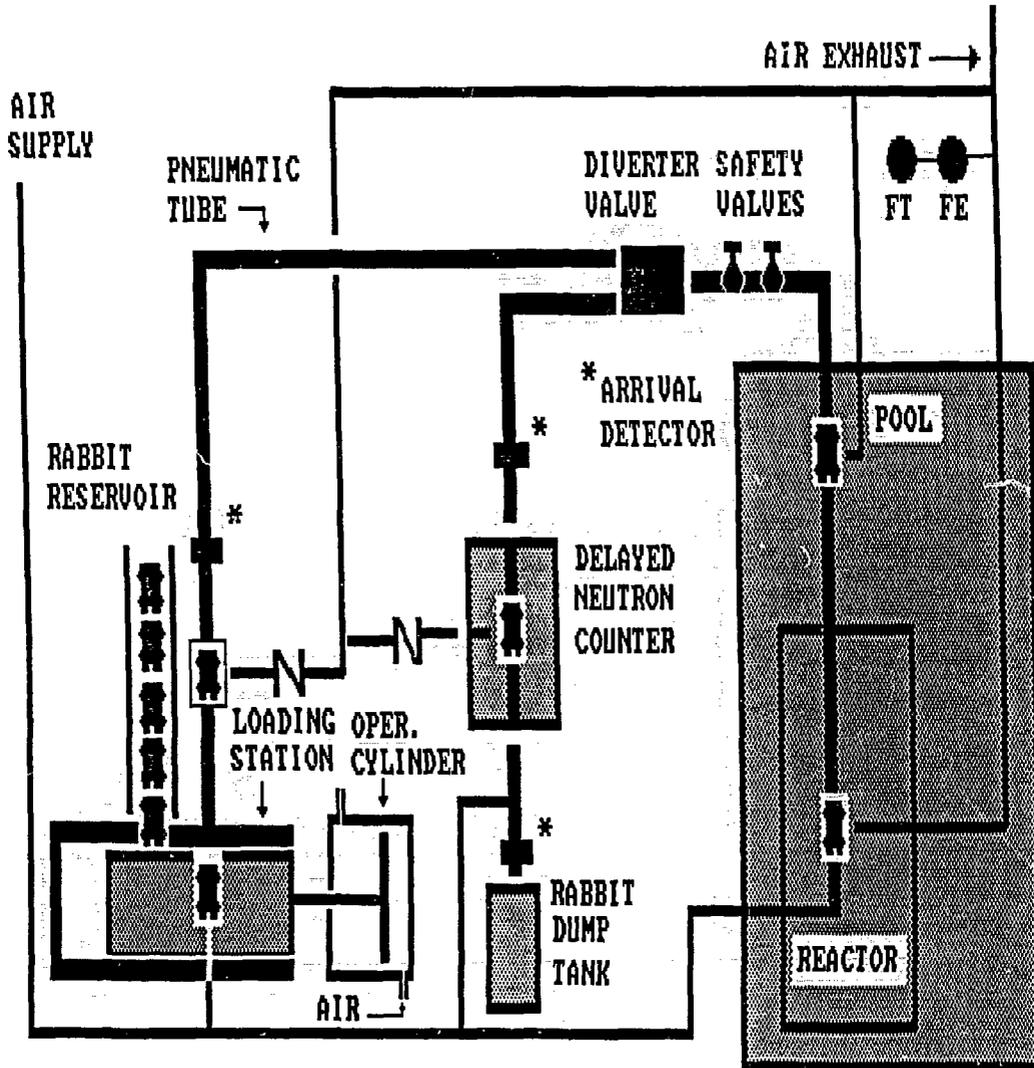
Fig. 2. Isometric drawing of first pneumatic tube of HFIR
