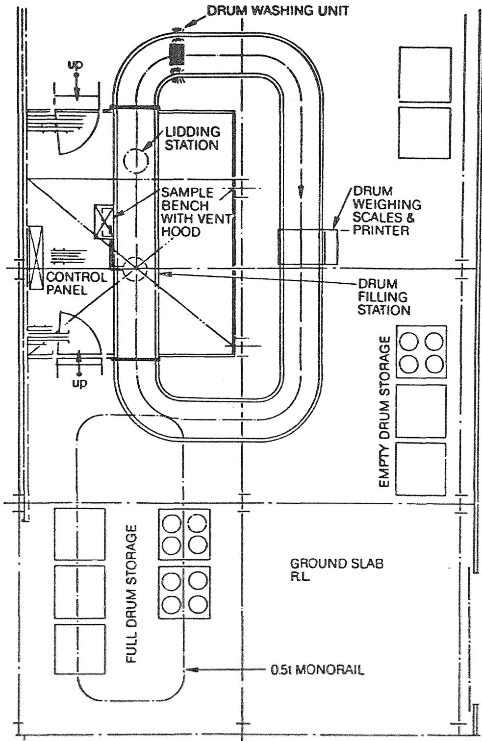
FIGURE 4: TYPICAL LAYOUT OF A PACKAGING AREA
