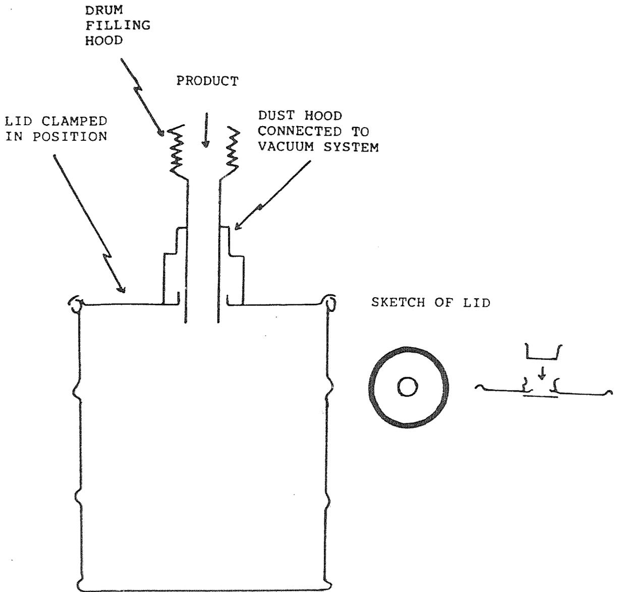
FIGURE 3: LIDS FOR AUTOMATIC CAPPING
