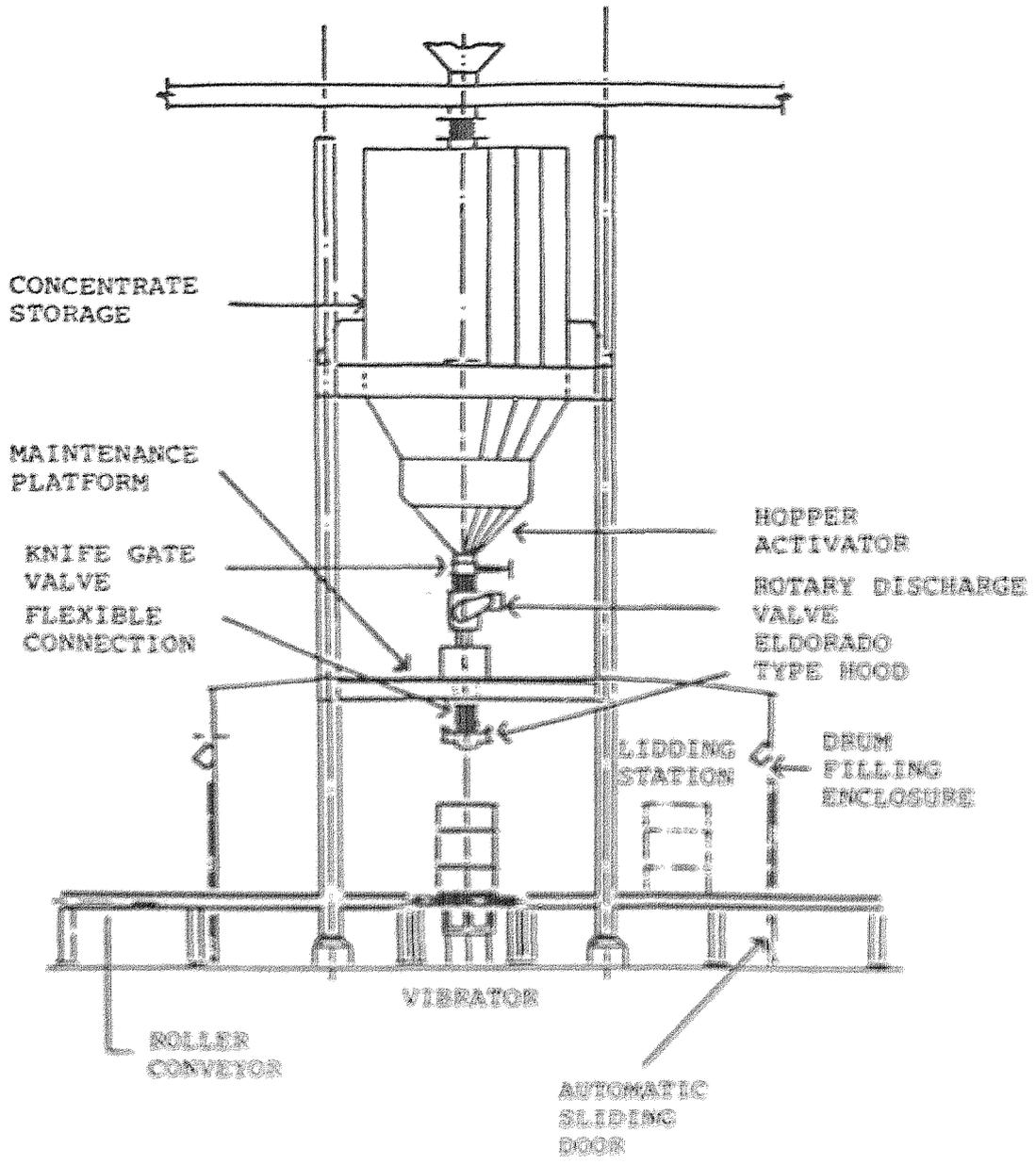
FIGURE 1: ELEVATION FOR PACKAGING AREA
