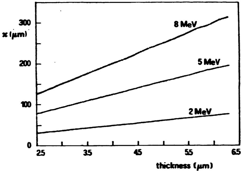
Fig. 14 Central peak wavelength as a function of dielectric thickness  $d$ , electron energy.
