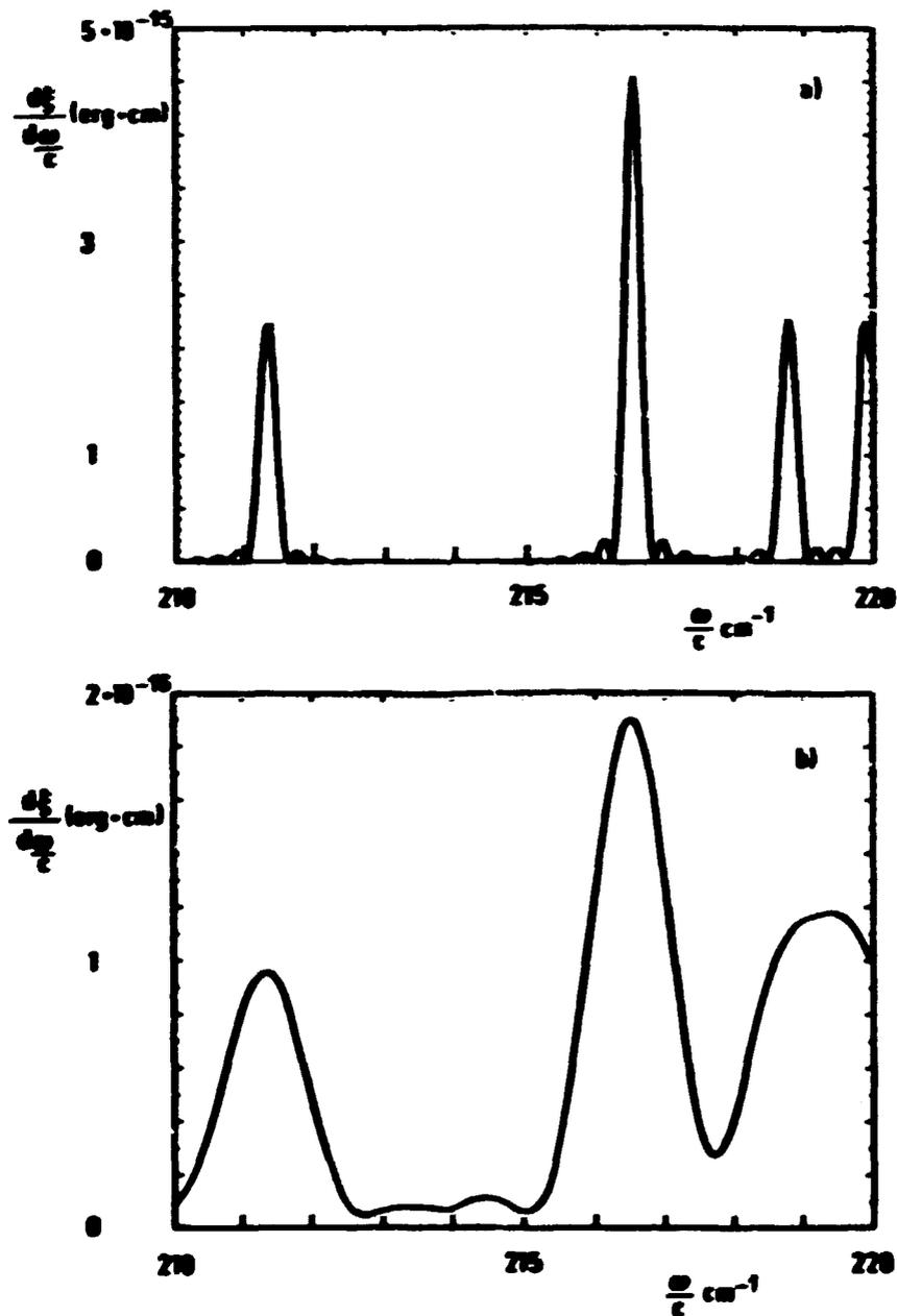
Fig. 7 On axis spectrum for a rectangular waveguide, only the odd modes are excited: (a) the excited modes are well distinguished ( $L=25 \text{ cm}$ ); (b) for shorter interaction length it's to be noted a remarkable interference ( $L=5 \text{ cm}$ ).
