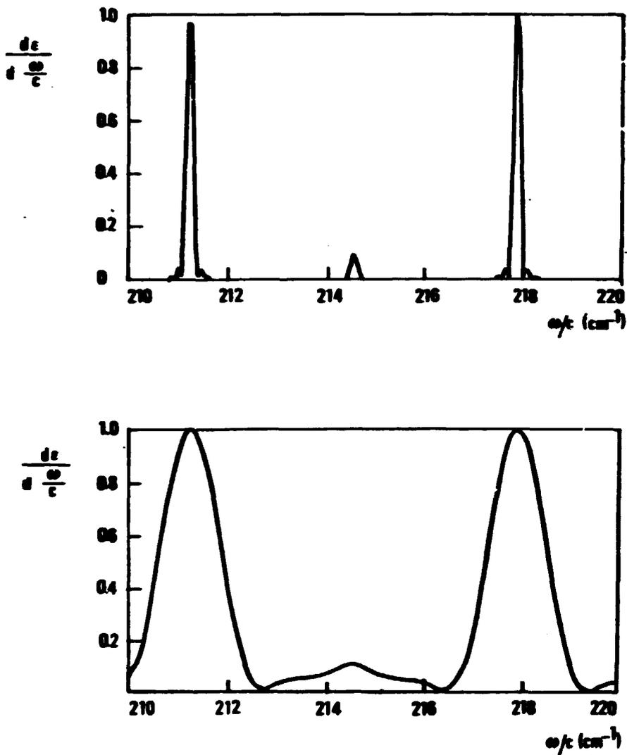
Fig. 4 Off-axis spectrum for a circular waveguide ( $\rho_0/a=0.01$ ). The number of excited modes is increased.
