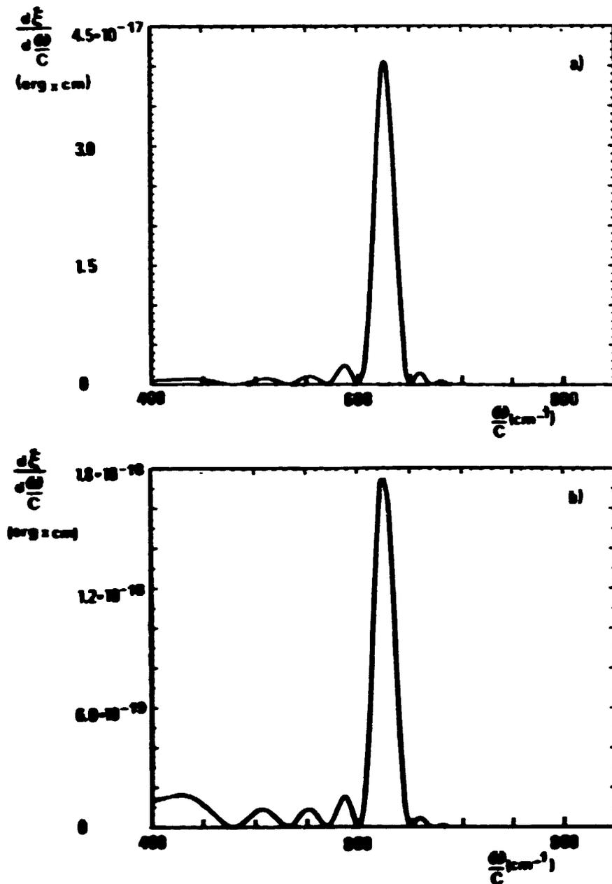
Fig. 13 Energy spectrum for the slab configuration ( $d=3.2 \mu\text{m}$ );
