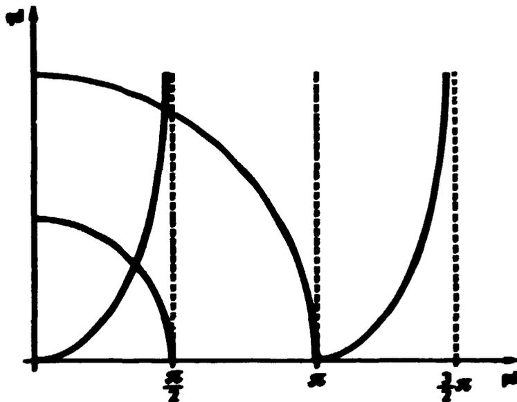
Fig. 12 The dispersion relations. The transverse wavenumbers  $p$  and  $q$  for  $\text{TM}_n$  mode are determined by the intersection between the circumference and the  $n$ -th branch of the circular tangent.
