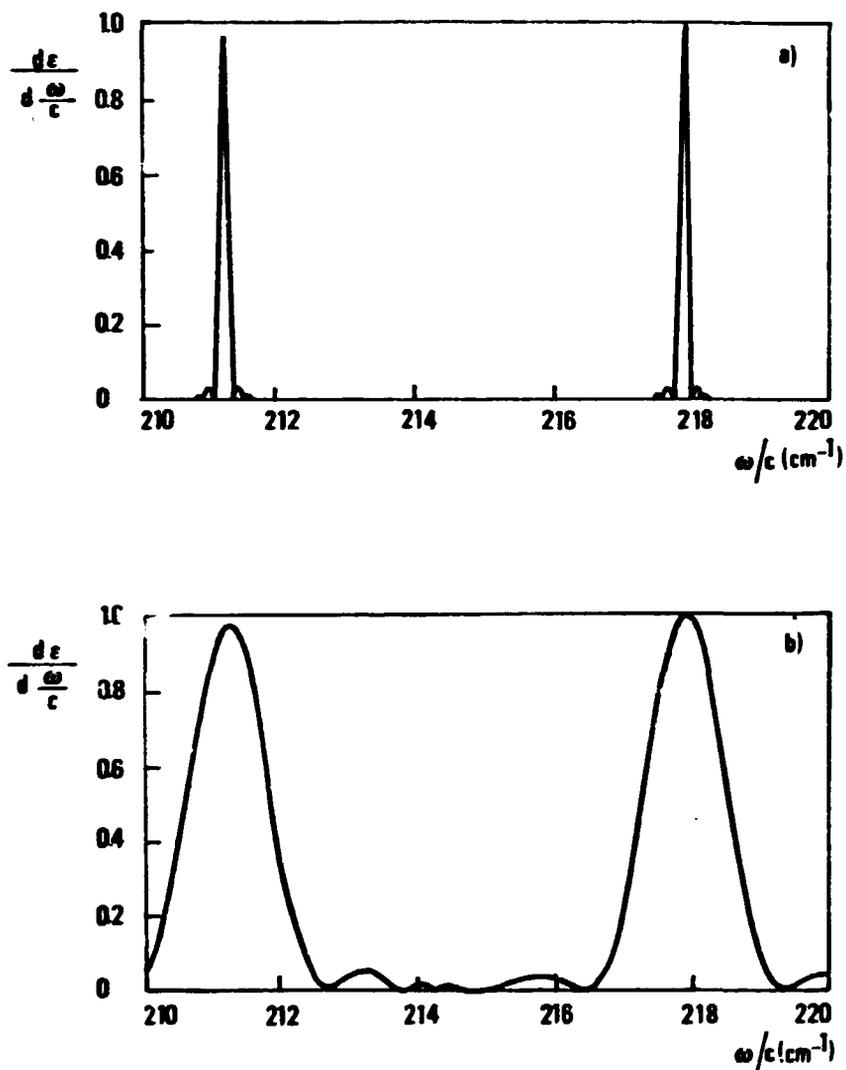
Fig. 3 On axis spectrum for a circular waveguide: (a) the sinc-functions are well distinguished ( $L=50$  cm;  $[d/d(\omega/c)]_{\max} = 0.89 \times 10^{-14}$  erg x cm); (b) for shorter interaction length an interference arises between the two modes ( $L=5$  cm;  $[d/d(\omega/c)]_{\max} = 0.90 \times 10^{-16}$  erg x cm).
