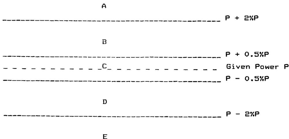
Fig-9 The control Band-width of the reactor power
