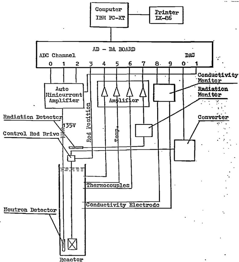
Fig.1 The block diagram of the control system
