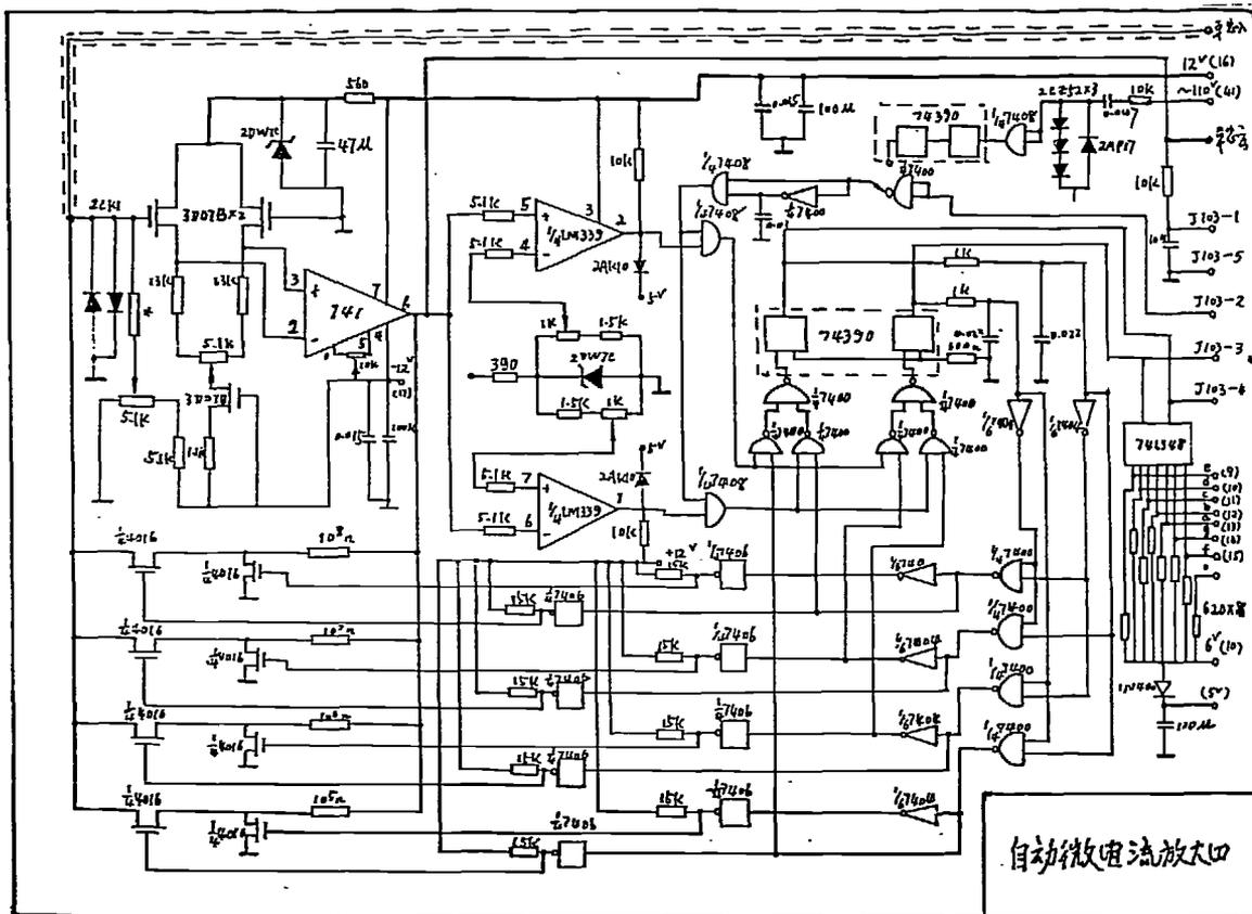
Fig.3 The circuit of the micro\_current amplifier
