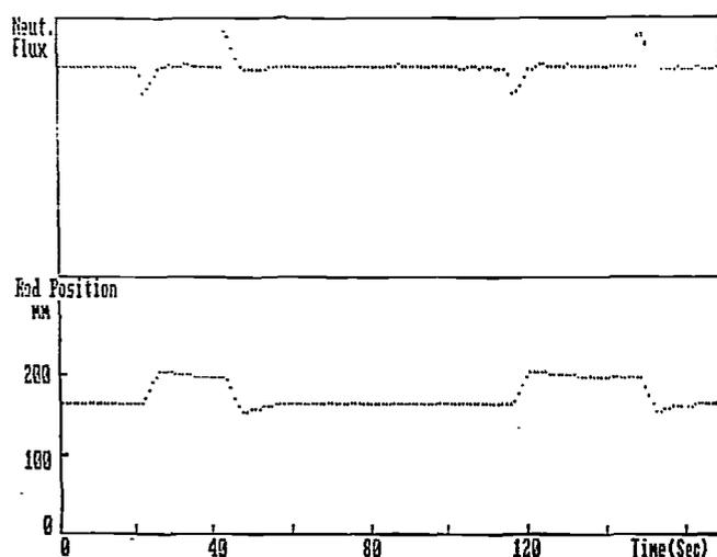
Fig.11 The response characteristic of the control system
