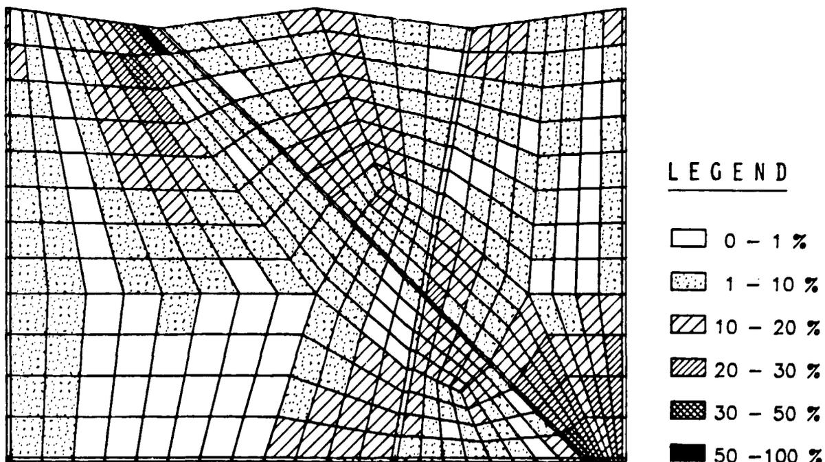
Fig. 16 Mass balance deviation index in Case 3.
