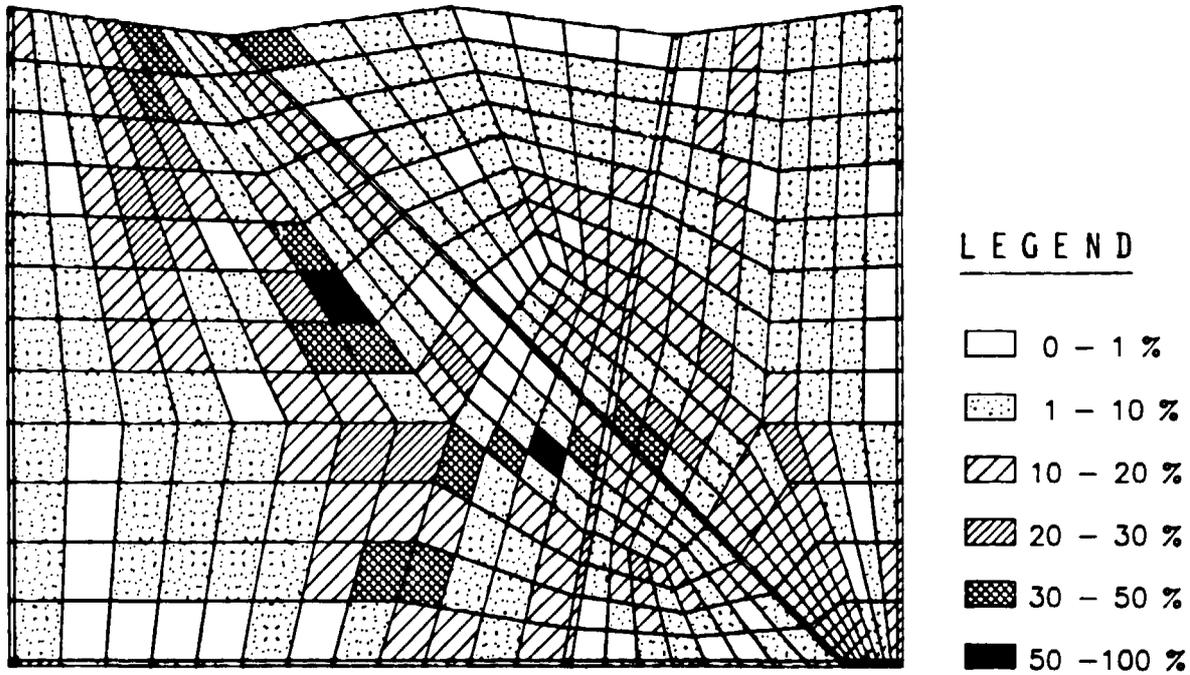
Fig. 18 Mass balance deviation index in Case 4.
