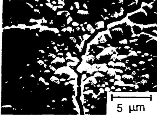
Figure 2: Surface of tungsten specimen after electron irradiation with 30 MeV for 30 s. The irradiation caused grain growth and microcracking (SEM micrograph)
