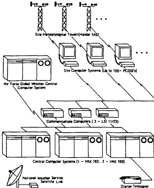
Fig. 1 A schematic diagram of the ARAC hardware system.
