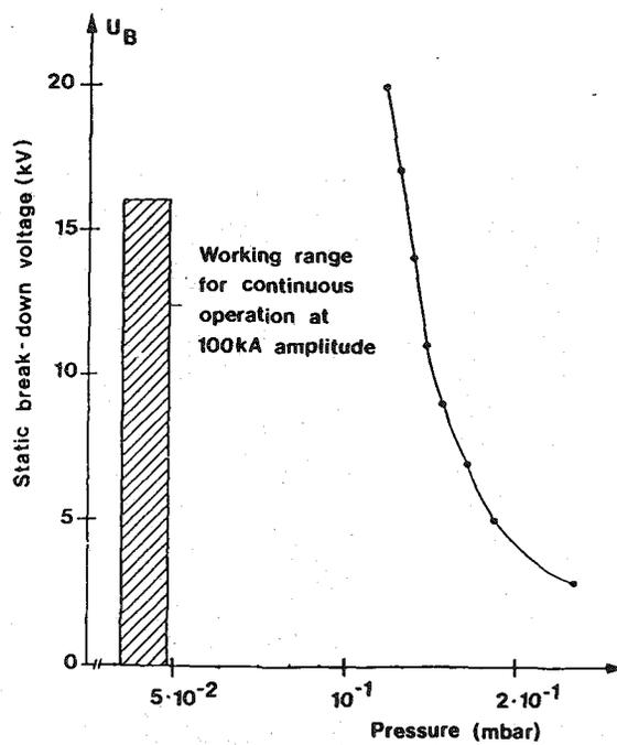
**Fig. 27** Static breakdown curve and operating range of the high-current pseudospark switch
