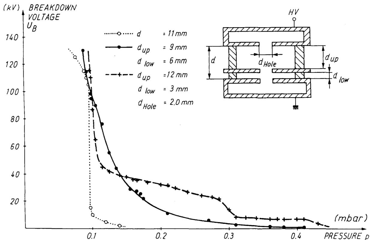
Fig. 33 Comparison of breakdown characteristics in a single-gap, high-voltage pseudospark switch with and without the intermediate electrode.
