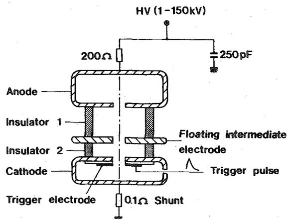
Fig. 32 Electrical scheme of the high-voltage pseudospark switch
