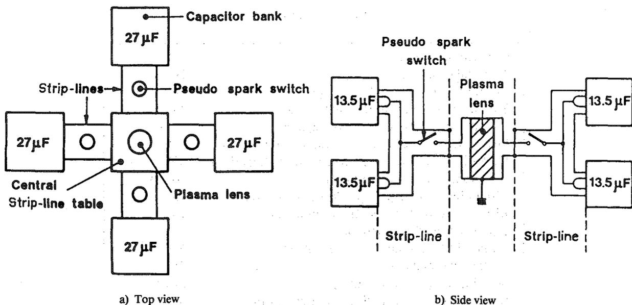
Fig. 21 Schema of the plasma-lens pulse generator
