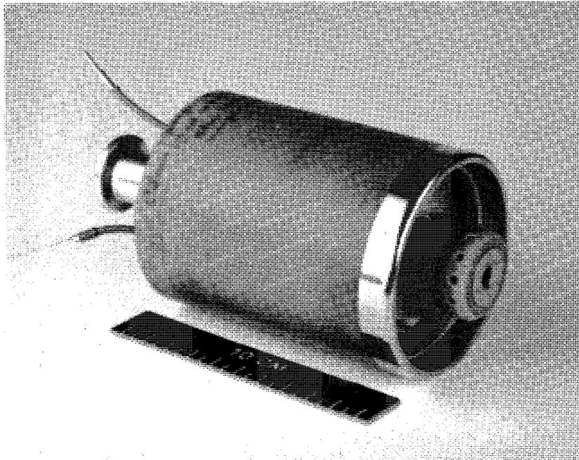
**Fig. 24** Modular charge injection trigger for the high-current switch
