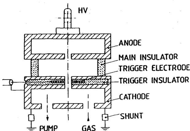
Fig. 7 Principle of a dielectric surface-discharge trigger
