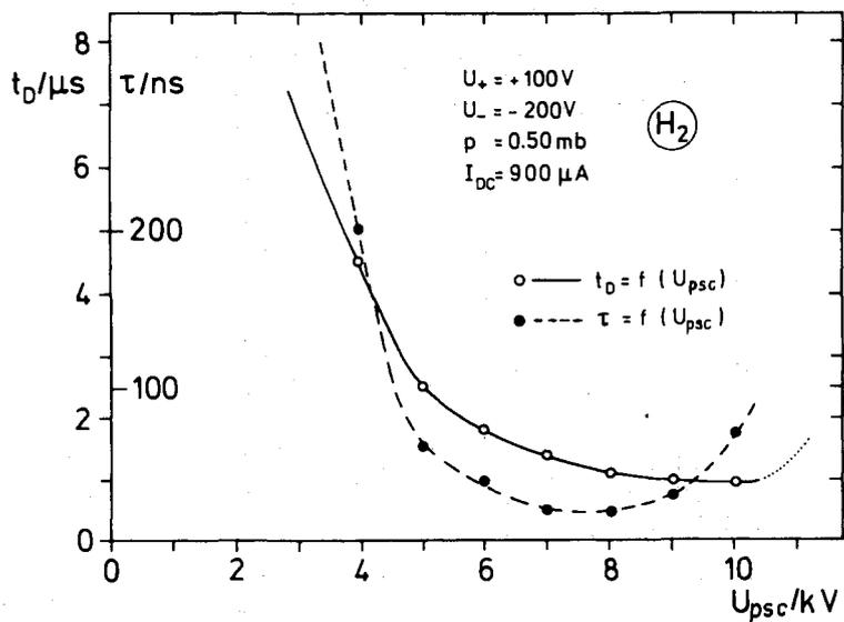
Fig. 11 Delay  $t_D$  and jitter  $\tau$  as a function of voltage  $U_{psc}$  for the continuous electron-beam trigger
