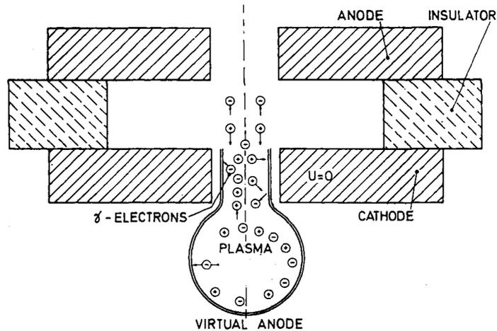
Fig. 5 Virtual anode formation in the hollow cathode of a pseudospark chamber.
