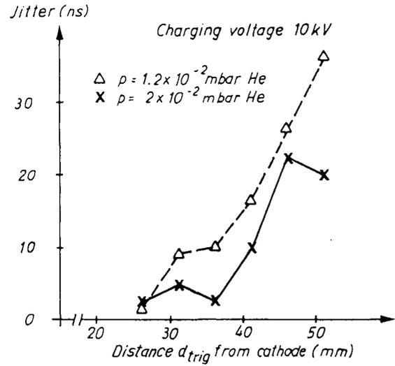
Fig. 18 Jitter of the high-current switch discharge at low surface-discharge trigger at low (1 J) pulse energy as a function of the trigger distance from the main gap
