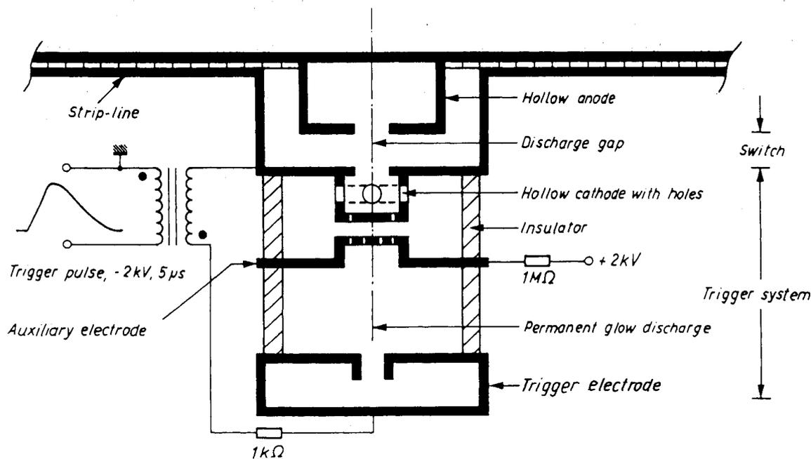
Fig. 14 Principle of a simplified charge-injection trigger for high-current pseudospark switches
