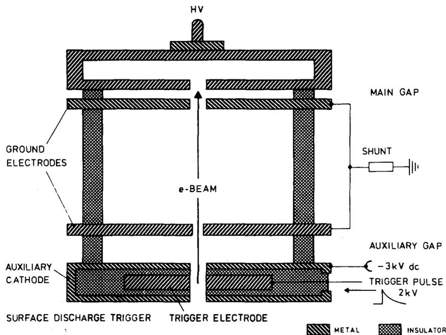
Fig. 12 Schema of a single-gap pulsed electron-beam trigger
