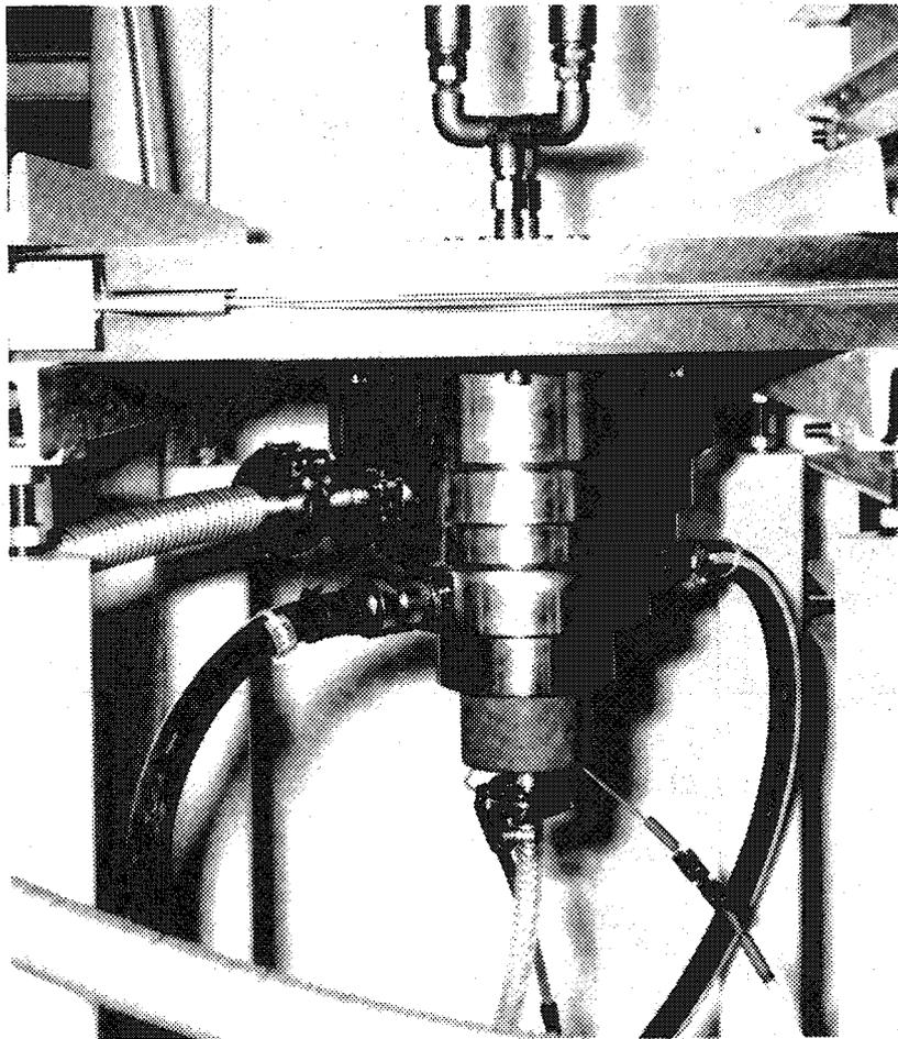
Fig. 22 High-current pseudospark switch mounted into the strip line of the plasma-lens pulse generator
