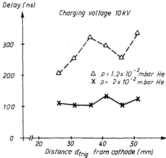
Fig. 17 Delay of the high-current pseudospark switch at low surface-discharge trigger at low (1 J) pulse energy as a function of the trigger distance from the main gap
