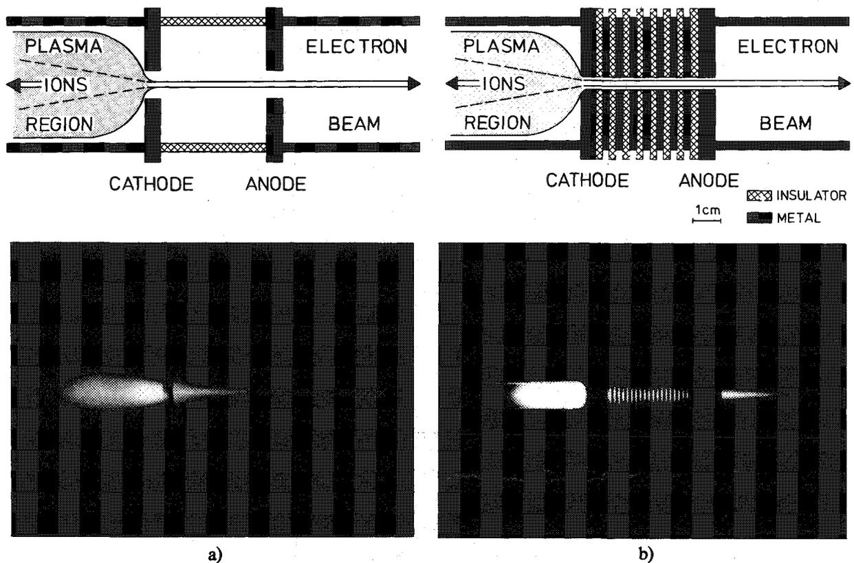
Fig. 4 Principle (top) and view (below) of a single-gap (a) and a multigap (b) pseudospark chamber
