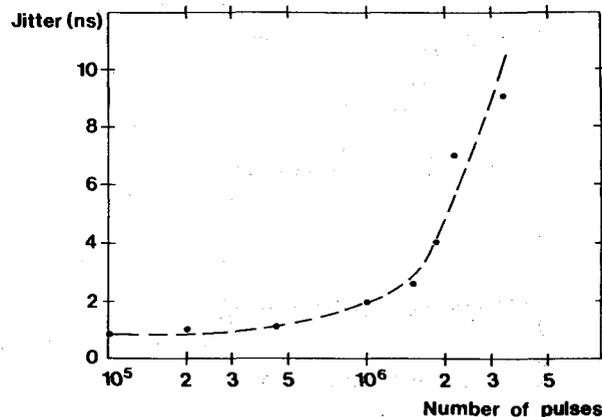
Fig. 15 Jitter as a function of the number of pulses for a pseudospark switch with a surface-discharge trigger switching 30 kV and 600 A and a 400 ns long pulse
