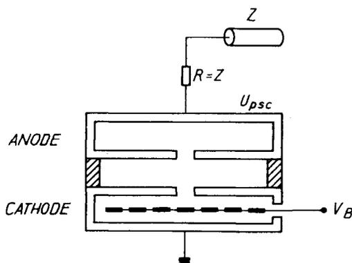
Fig. 9 Switching of a pseudospark switch by a blocking-electrode potential ( $V_B$ ) commutation. Charging voltage =  $U_{psc}$ .
