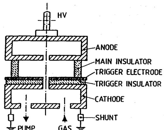
Fig. 8 Diagram of the surface-discharge trigger with the trigger electrode inside the main gap (highest possible switching precision!)
