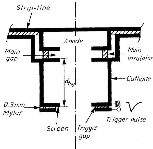
**Fig. 16** Schema of the surface-discharge trigger for the high-current switch
