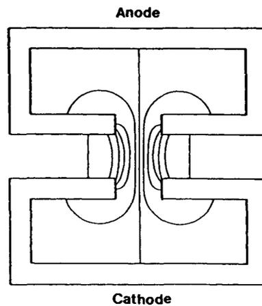
Fig. 6 Diagram of current flow in a single-gap pseudospark chamber
