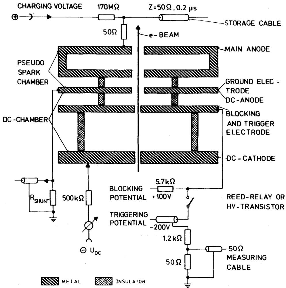
Fig. 10 Principle of the continuous electron-beam trigger
