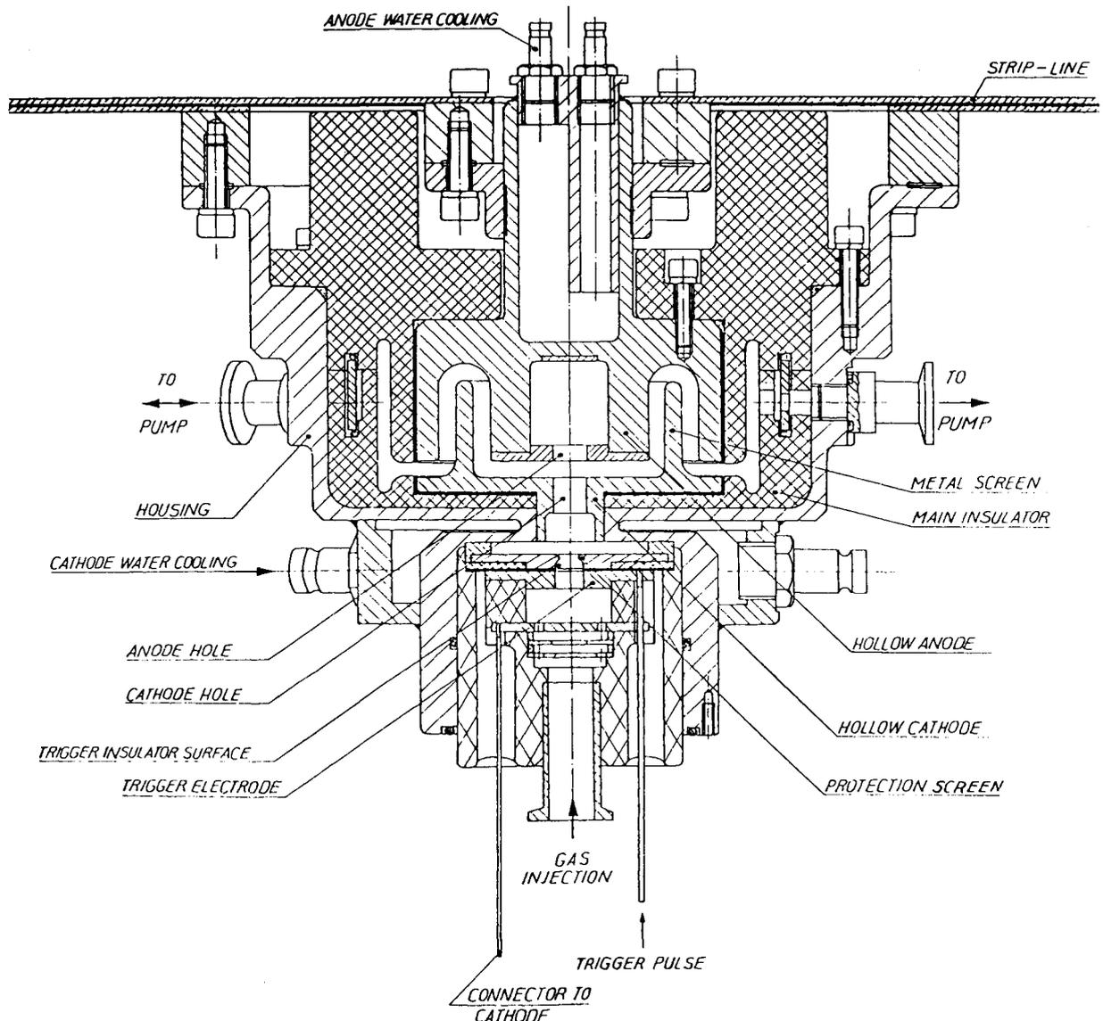
Fig. 19 Mechanical layout of the CERN high-current pseudospark switch
