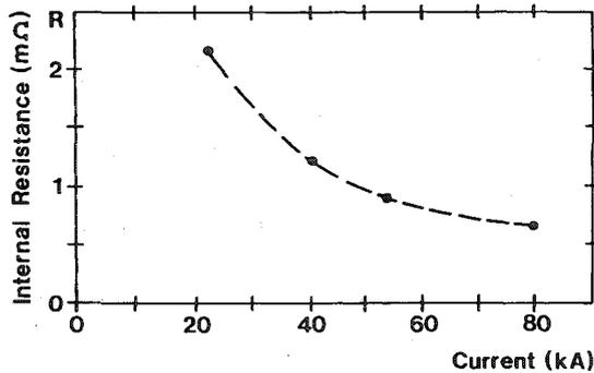
Fig. 30 Internal resistance of the high-current switch at peak current ( $di/dt = 0$ ).
