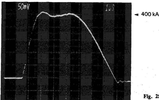
Fig. 25 Total plasma-lens current = sum of four pseudospark switch currents
