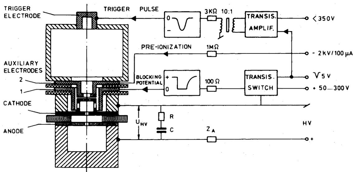
Fig. 13 Schema and electrical circuit of the charge-injection trigger (from Ref. [18])
