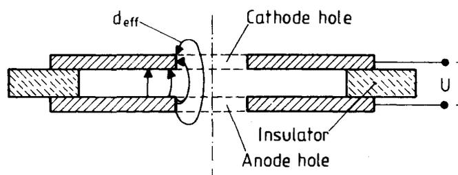
Fig. 2 Basic scheme of a single-gap pseudospark chamber
