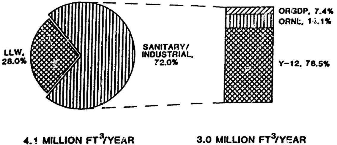
Fig. 2. Solid LLW and sanitary/industrial waste generated on the ORR in CY 1986, showing breakdown, by plant, of the sanitary/industrial waste portion.
