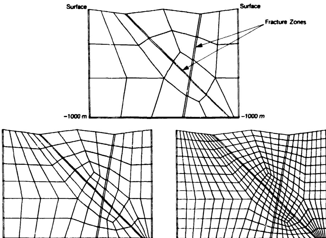
**Figure 6.** For solving the equations a mathematical method called the finite elements method is often used. The modelled domain is divided into a network of elements and the equations are solved by approximations within each element. The figure show a set of finite element networks (*meshes*) at three different levels of detail. (HYDROCOIN Level 1, case 2). The finest network will give the most accurate solution but it will also require more computer time.
