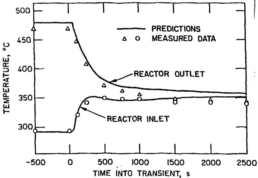
Figure 6. Loss-of-Heat-Sink Without Scram Test in EBR-II
