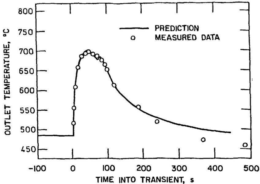
Figure 5. Loss-of-Flow Without Scram Test in EBR-II
