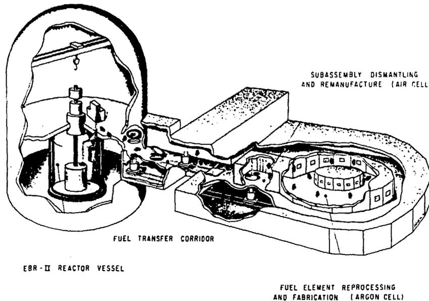
Figure 1. EBR-II Reactor and Fuel Cycle Facility
