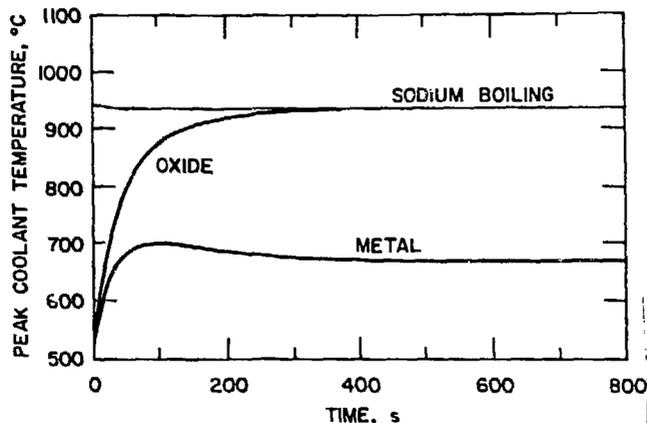
Figure 4. Loss-of-Flow Without Scram for Large Reactors (1350 MWe)
