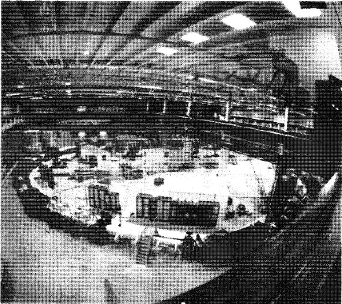
**Plate 4** A view of the AA ring. The coaxial lines linking stochastic cooling pick-ups and kickers can clearly be seen.
