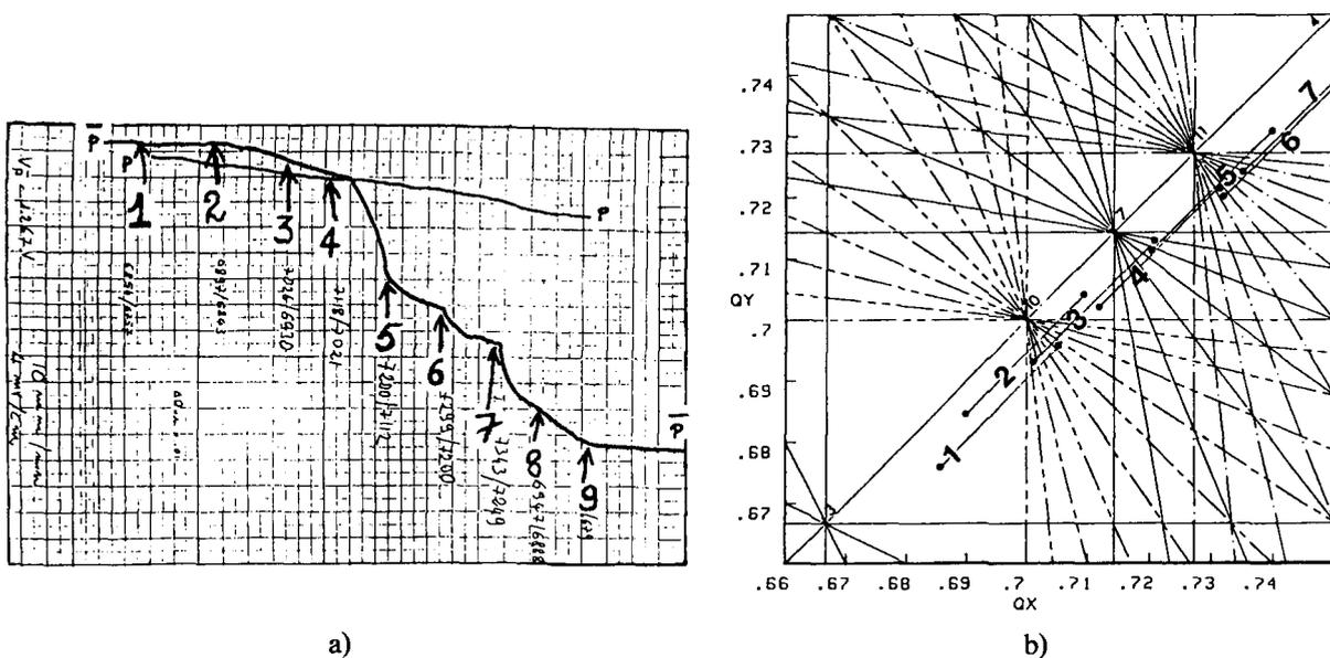
**Fig. 4** The beam-beam effect in the SPS. (a) A chart recorder output of the intensity decay (zero suppressed) of a strong proton bunch colliding with a weak antiproton bunch as the working point (b) is varied.
