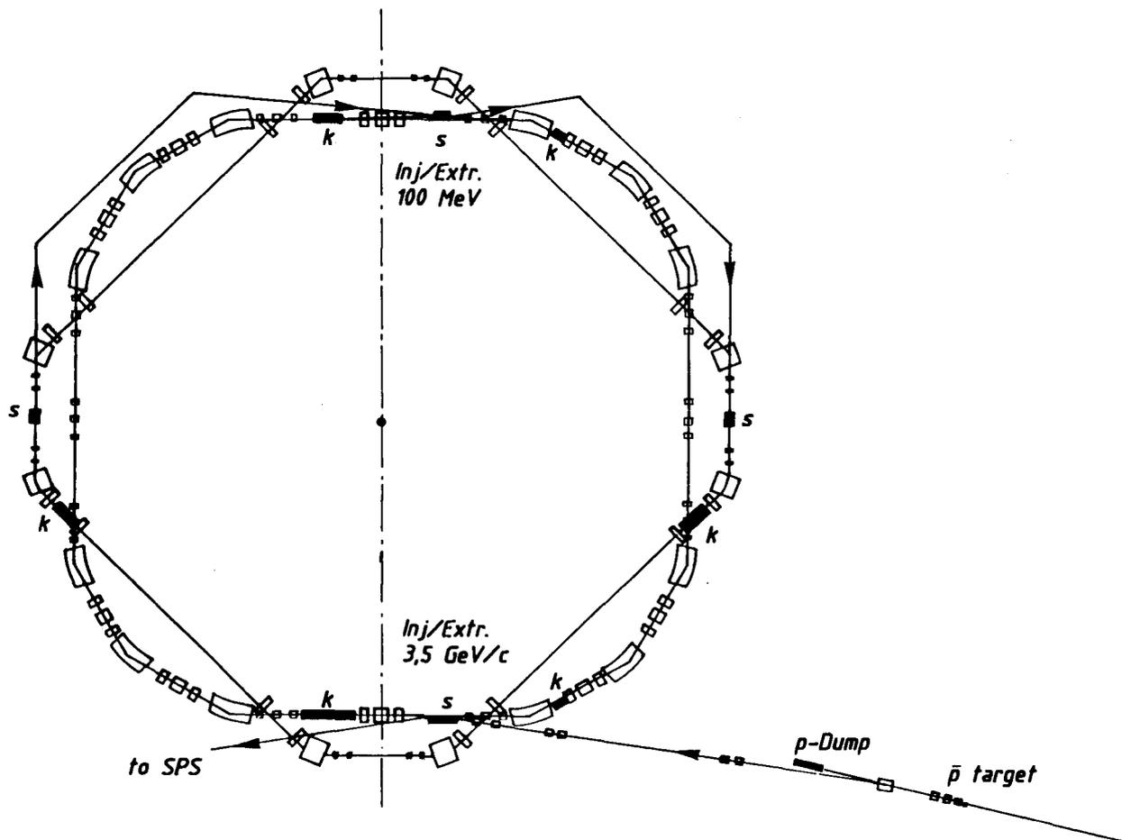
Fig. 2 The first proposal for an antiproton source consisted of a 3.5 GeV ring (shuttle ring) for bunch rotation and deceleration and a 100 MeV cooling ring using electron cooling
