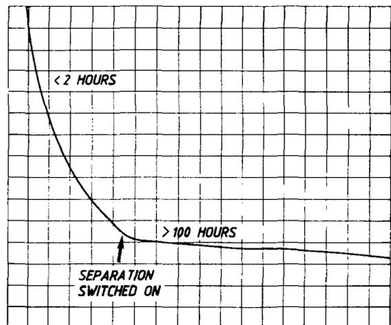
Fig. 6 Chart recorder output of the intensity decay of a single antiproton bunch in the presence of 6 dense proton bunches (zero suppressed) as separation is switched on.
