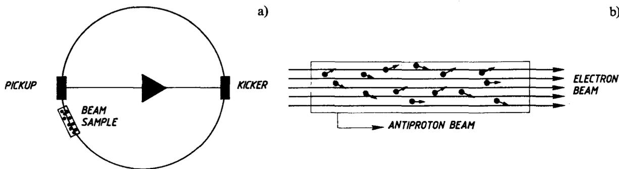
Fig. 1 (a) Stochastic cooling and (b) electron cooling
