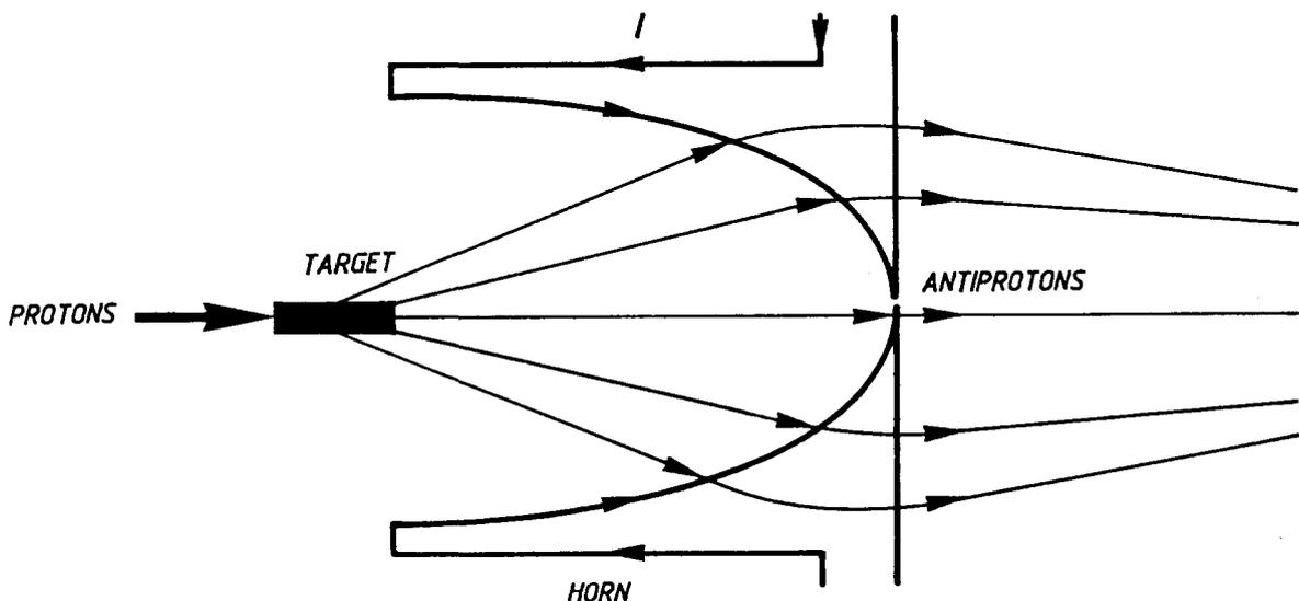
Fig. 3 Focusing horn for antiproton production
