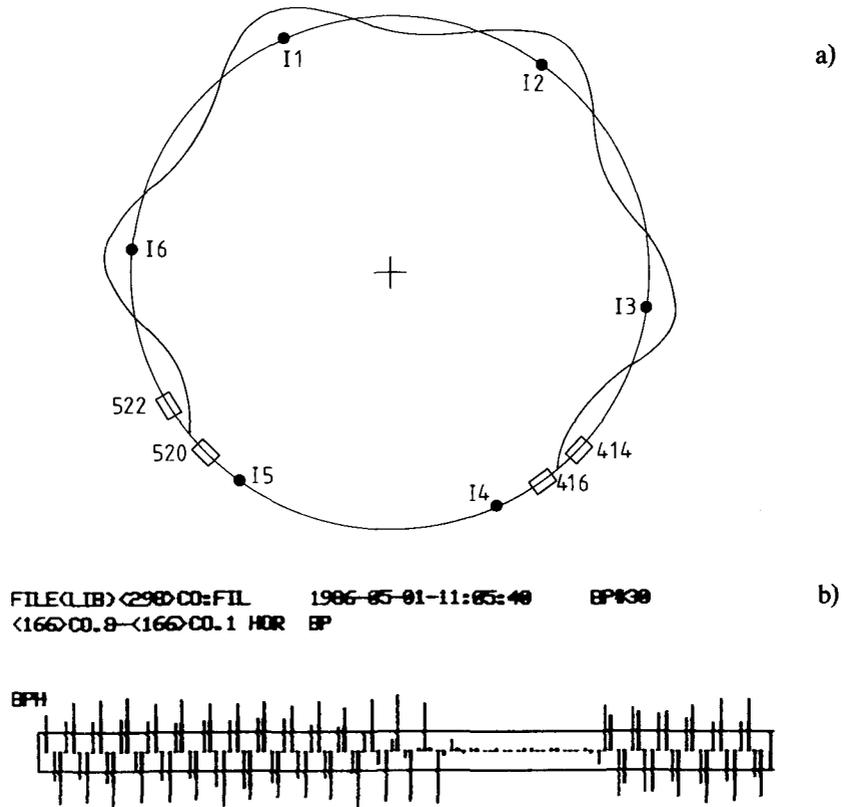
Fig. 5 Beam separation using electrostatic deflectors. (a) Schematic of SPS separation scheme with electrostatic deflectors. (b) Measured closed orbit with separation.
