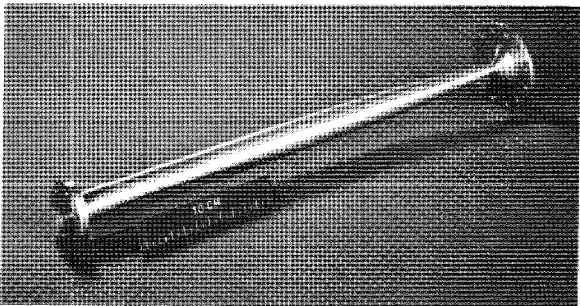
**Plate 5** The inner conductor of the coaxial horn for the focusing of antiprotons from the target.
