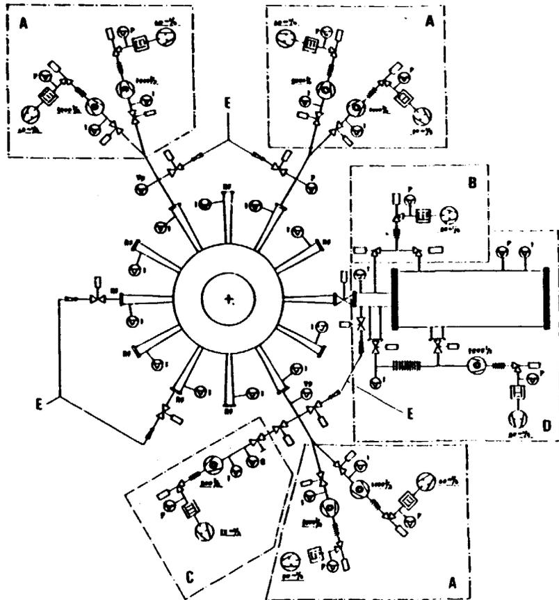
**Fig. 3 FTU vacuum system: A) Pump units; B) Roughing pump unit; C) Residual gas Analysis system; D) Limiter extraction chamber; E) Gas immission lines.**
