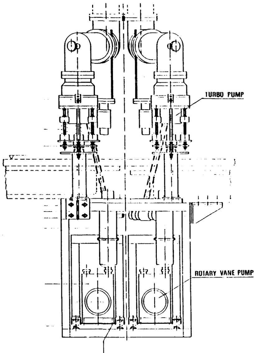
**Fig. 4 Pump units connection to a torus ports**
