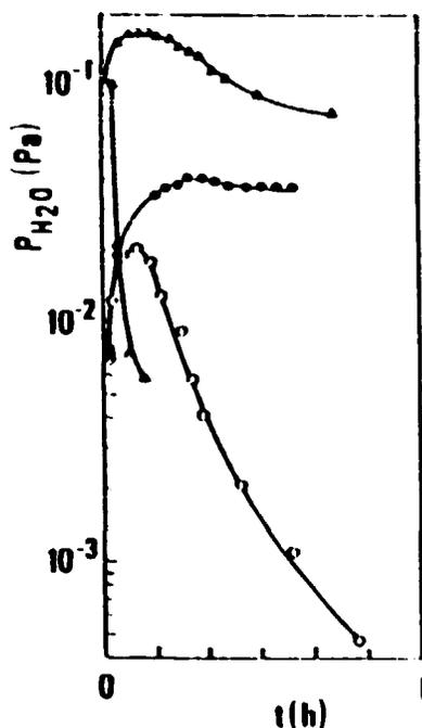
Fig. 7 Water partial pressure during dc;  $I_{DC} = 100$  mA.
