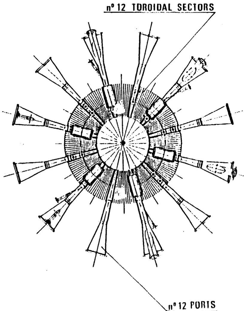
Fig. 1 FTU vacuum vessel
