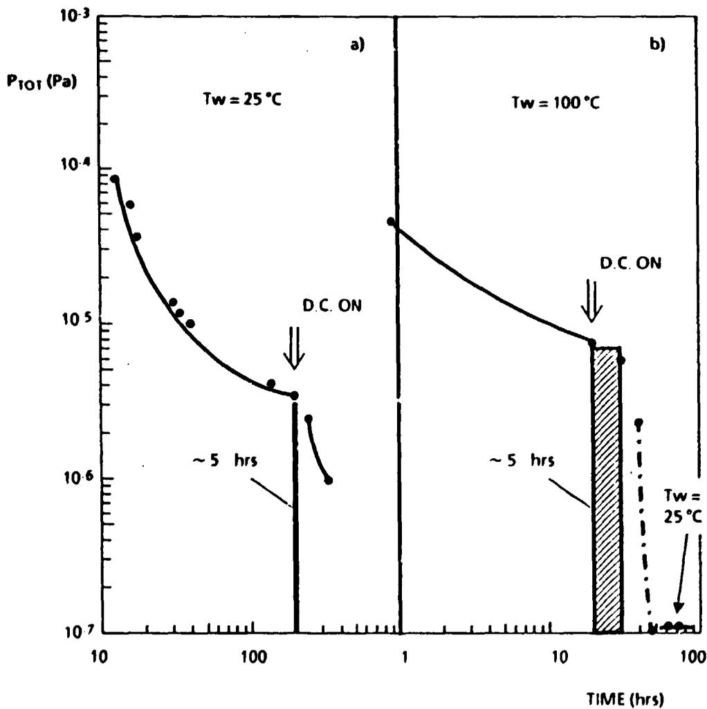
Fig. 6 Effectiveness of glow discharge vs wall temperature
