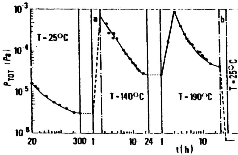
Fig. 5 Pressure vs time evolution during thermal outgassing.
