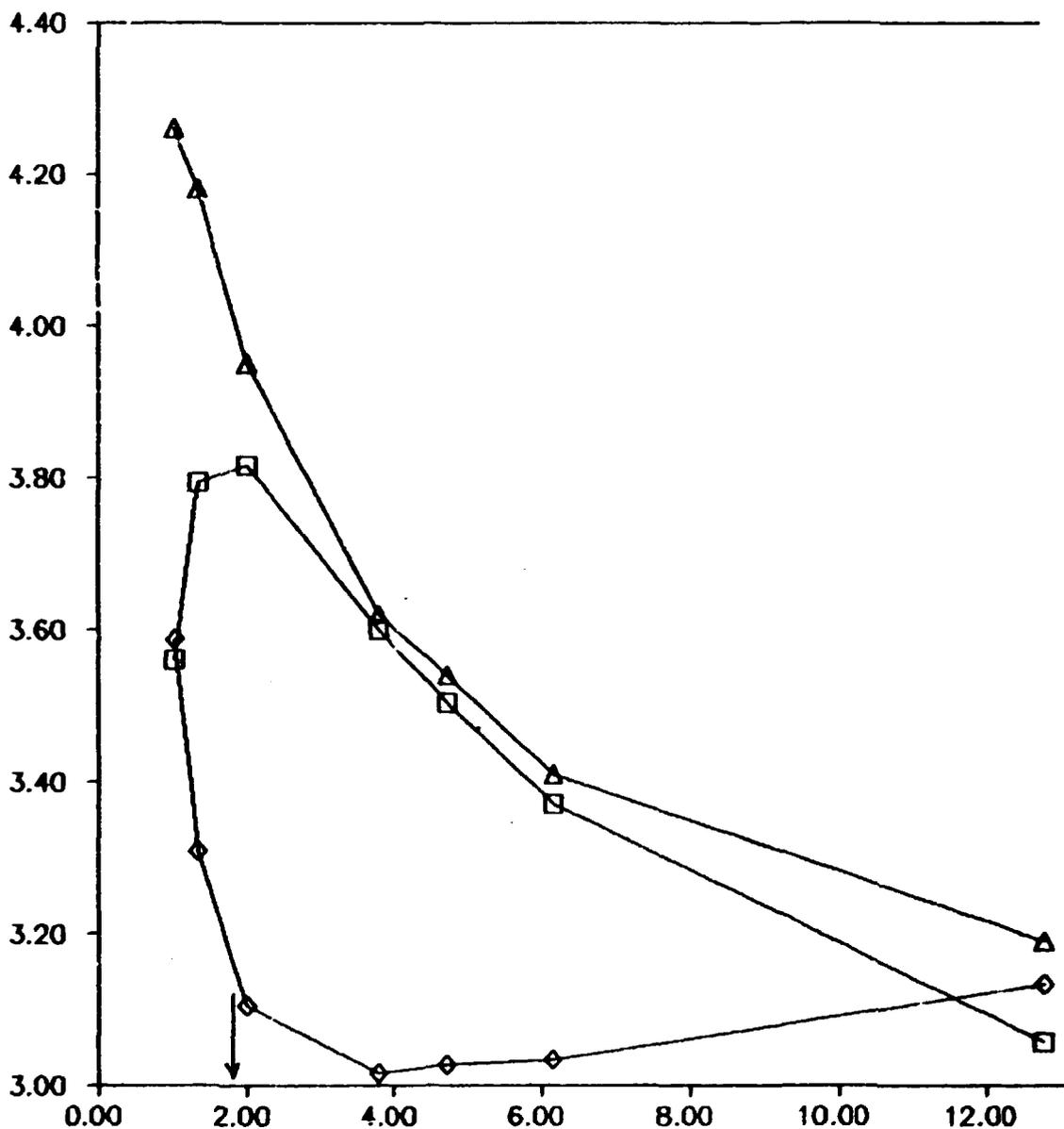
Fig. 4:  $3 \times$ mass, radius and  $R/m(R)$  versus central mass density for the Walecka equation of state with canonical values of the coupling constants (Walecka, 1974). Mass and radius in kilometers,  $\epsilon_0/c^2$  in  $10^{15}$  g/cm<sup>3</sup>. Symbols as on Fig. 1.
