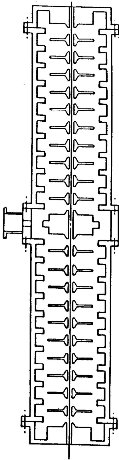
Figure 2: Disk-and-washer structure and  $\beta\lambda/2$  coaxial coupler (after a sketch of the LASL FIGMI proposal)
