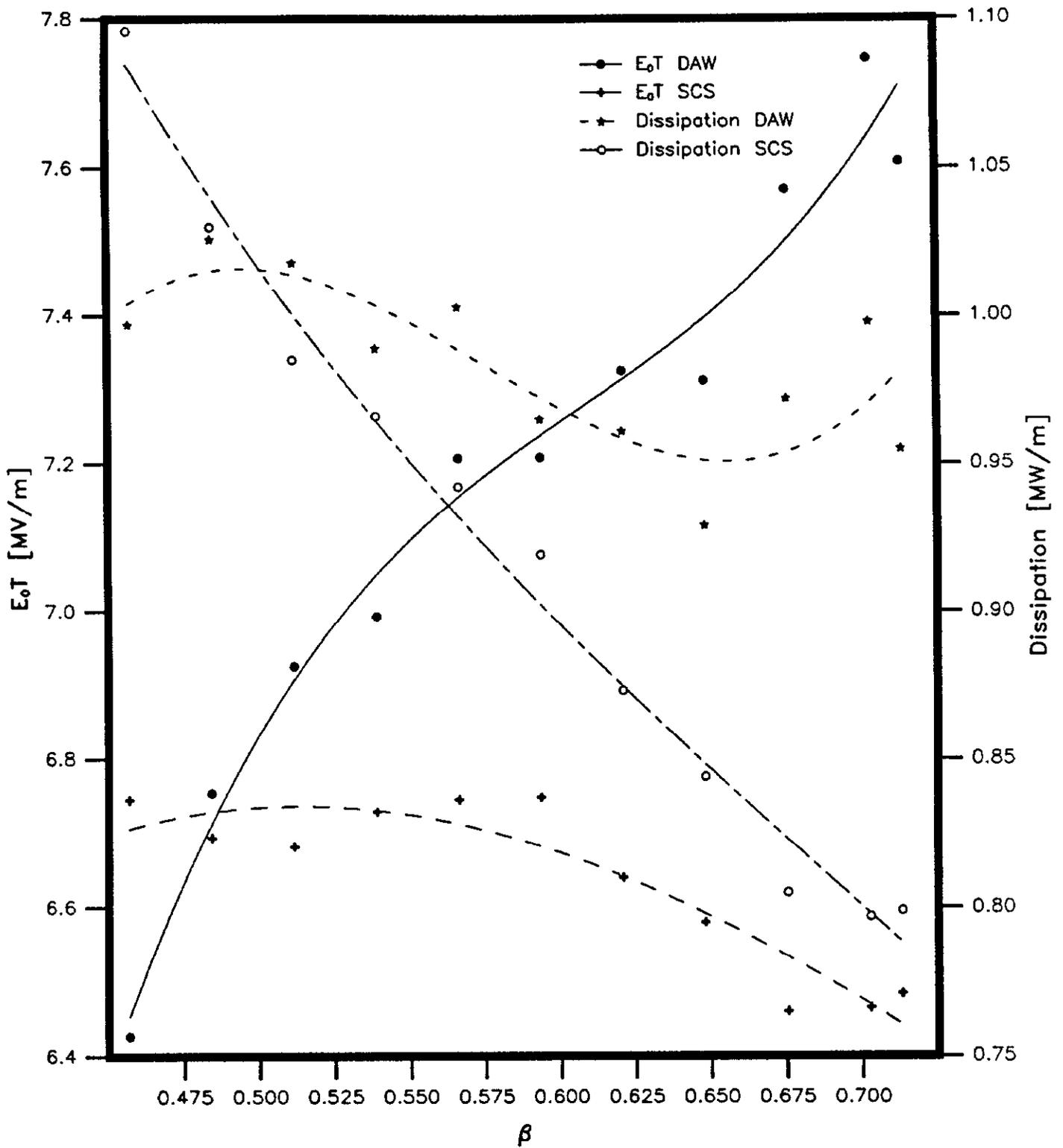
Figure 3: Third order least squares fits to effective accelerating gradient  $E_0T$  and power dissipation per meter for  $E_{max} = 42$  MV/m for both DAW and SCC as functions of  $\beta$
