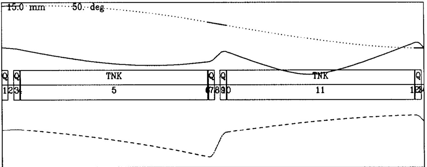
Figure 10: Beam envelopes in the transition section to the SCC Doublet-focussed Linac
