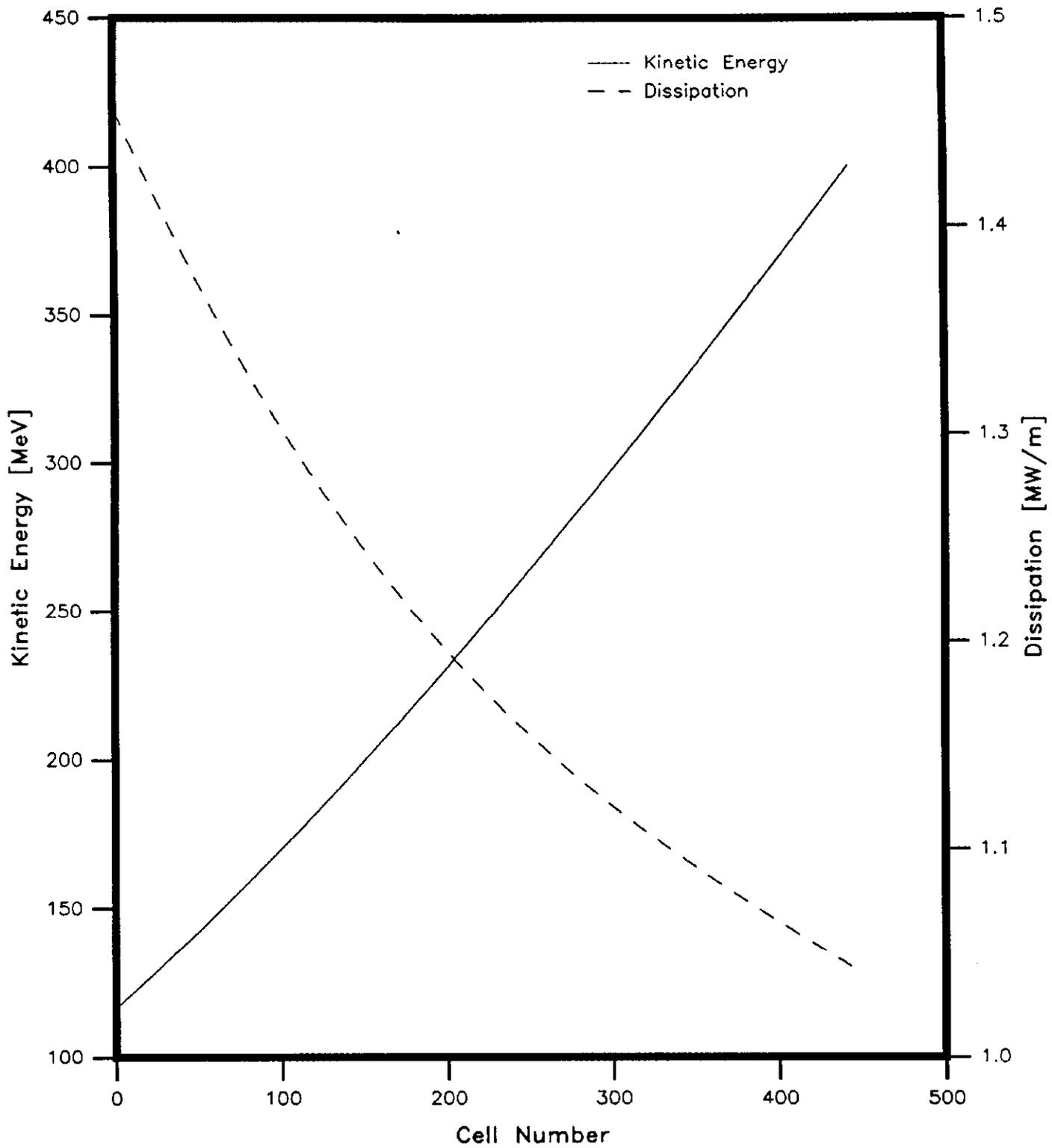
Figure 4: Kinetic energy and power dissipation per meter as functions of cell number
