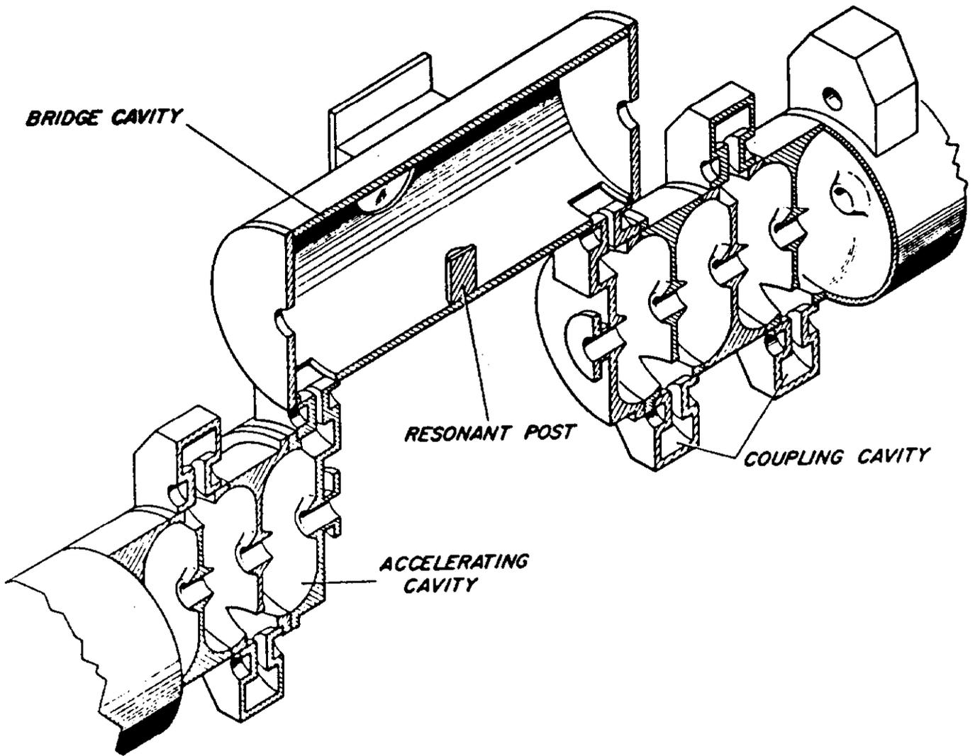
Figure 1: Side-coupled cavity structure and  $\frac{3}{2}\beta\lambda$  bridge coupler (after E. A. Knapp in *Linear Accelerators*, Lapostolle and Septier, ed., p615, North Holland(1970)
