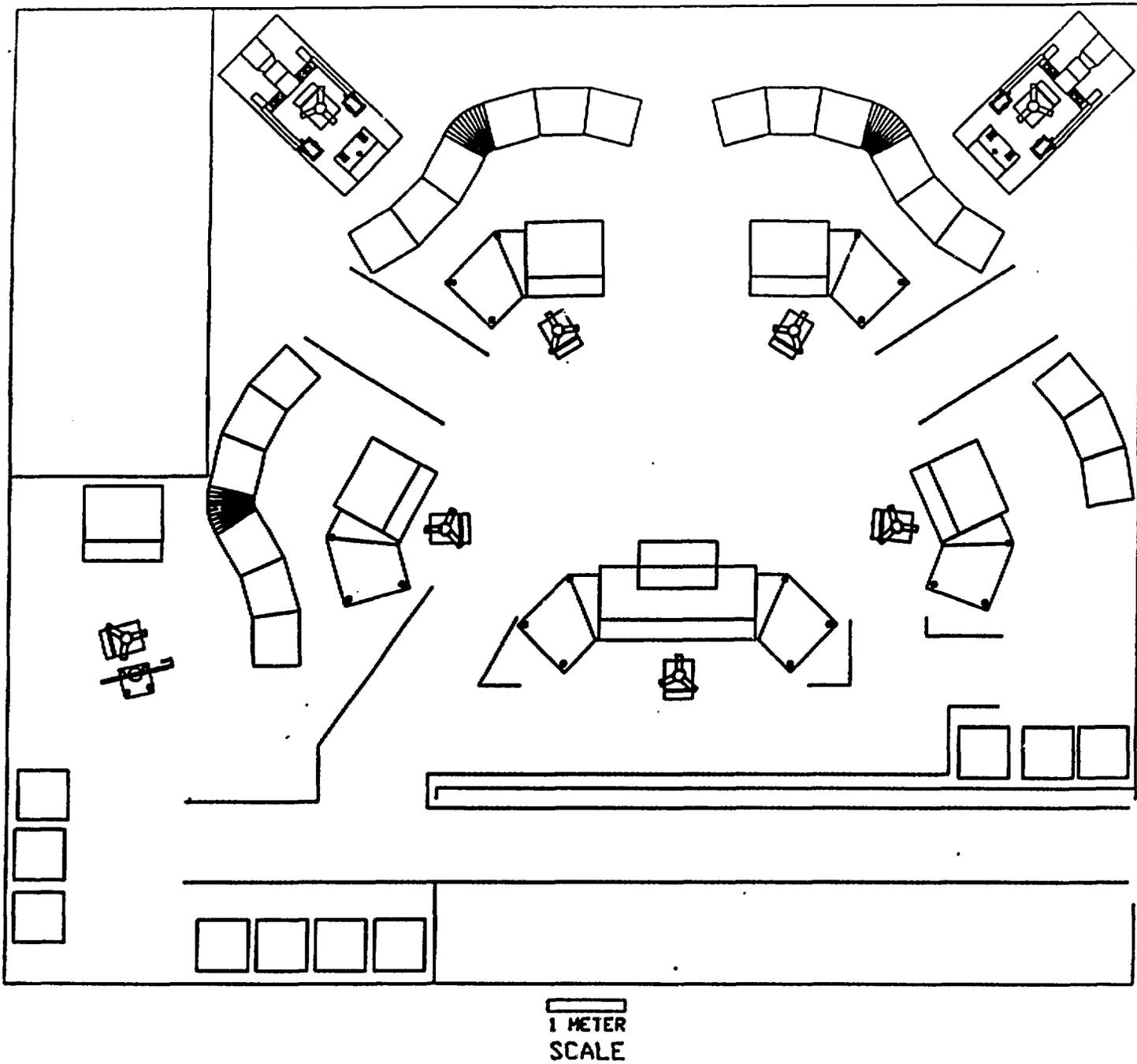
Fig. 1. Plan view of control room concept.
