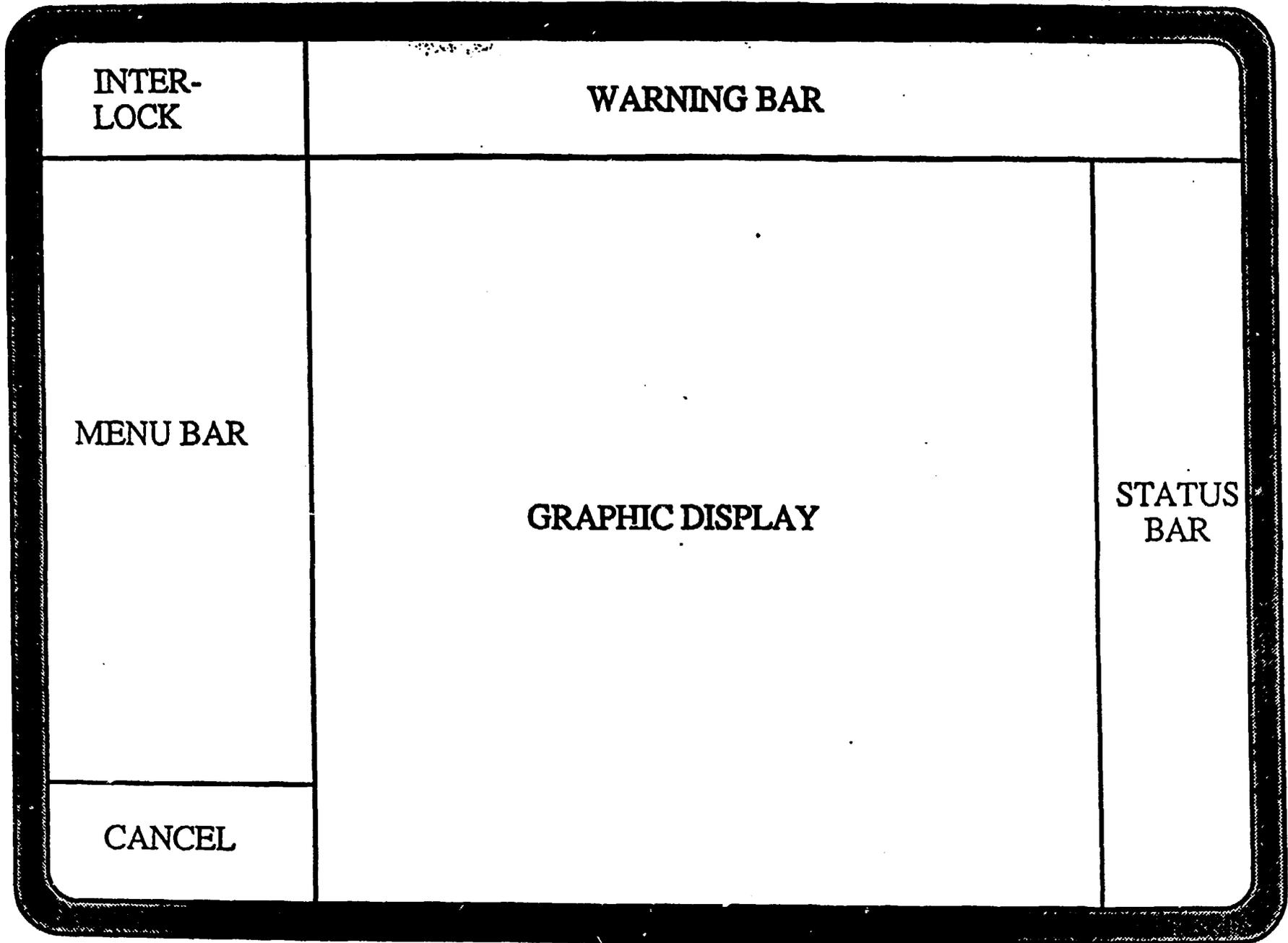
Fig. 5. Graphic screen arrangement,
