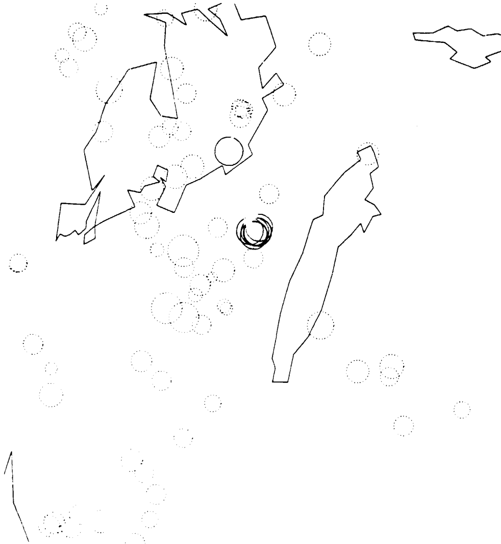
Figure 7. The epicenters of the earthquakes in the lake Vaenern area. The size of the circles are proportional to the focal depths. The solid circles belong to events of table 1.
