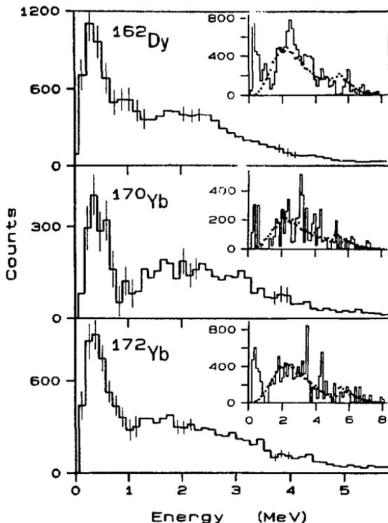
Figure 6.3: First-generation  $\gamma$ -ray spectra for  $^{162}\text{Dy}$ ,  $^{170}\text{Yb}$  and  $^{172}\text{Yb}$ , measured with NaI detectors. The corresponding excitation energy region is  $\approx 5.6 - 8.2$  MeV. Insert: Comparison between the unfolded experimental spectra (solid line) and the modified Fermi-gas model prediction (dotted line).
