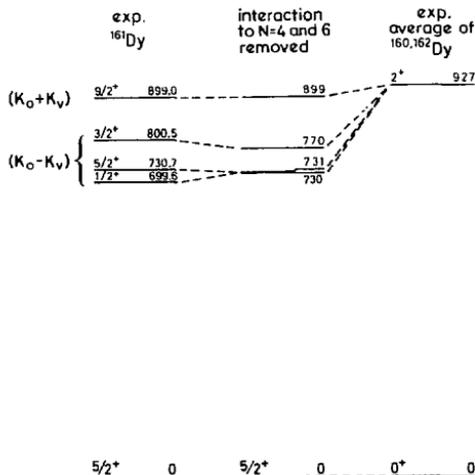
Figure 6.4: Experimental level scheme for excited  $K_0 \pm K_\gamma$  states in  $^{161}\text{Dy}$ . The middle part shows the unperturbed energies of the vibrational states when their interaction with the  $N = 4$  and 6 states have been removed.
