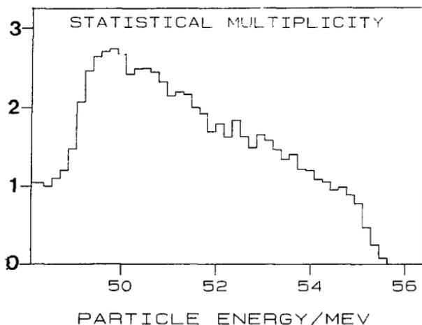
Figure 6.14: Gamma-ray multiplicity ( $E_\gamma > 0.43$  MeV) as a function of excitation energy in  $^{171}\text{Yb}$ .
