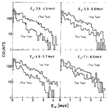
Figure 6.2: Spectra of  $\gamma$ -rays from the  $^{163}\text{Dy}(\tau, \alpha)$  and  $^{162}\text{Dy}(\tau, \tau')$  reactions measured in coincidence with ejectiles from four ranges of excitation energies in  $^{162}\text{Dy}$ .
