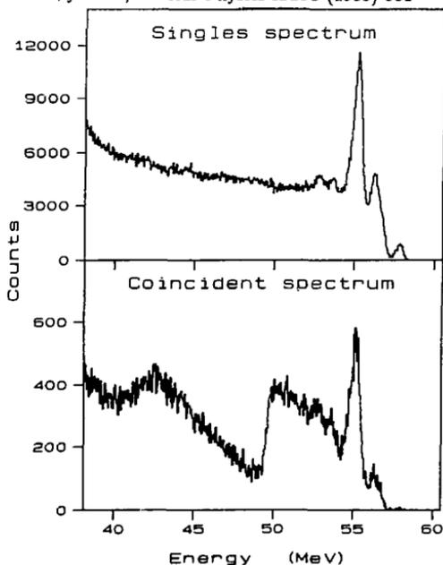
Figure 6.9: The  $\alpha$ -particle singles (top) and  $\gamma$ -coincident (bottom) spectra for the  $^{173}\text{Yb}(^3\text{He},\alpha)$  reaction.
