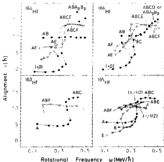
Figure 6.15: Experimental alignment  $i_z$  as a function of rotational frequency for  $^{163-166}\text{Hf}$ .
