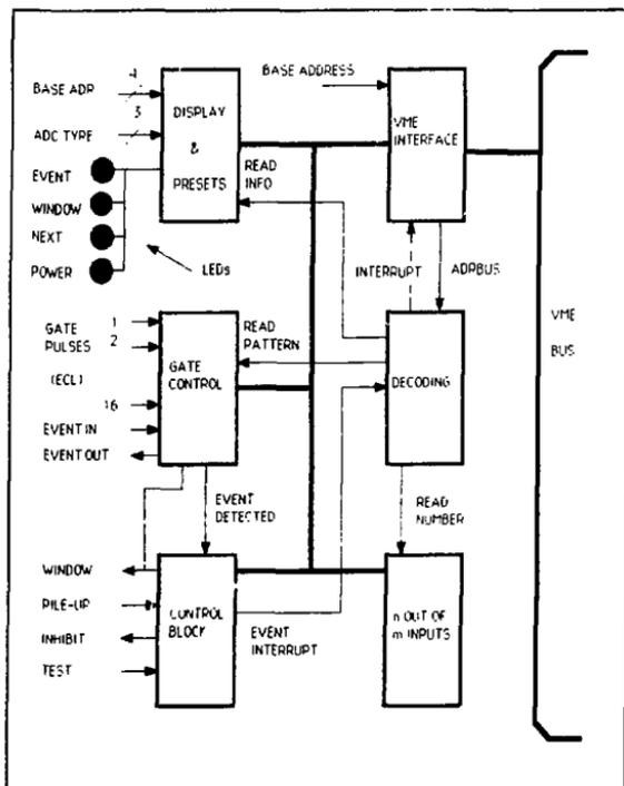
Figure 4.2: Trigger Pattern Unit (Master)
