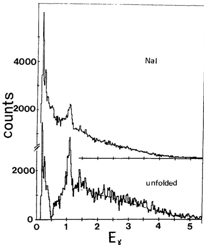
Figure 6.6: The NaI  $\gamma$ -ray spectrum from the  $E_x = 2.3 - 8.0$  MeV region. In the lower part the same spectrum unfolded with the NaI response function is shown.
