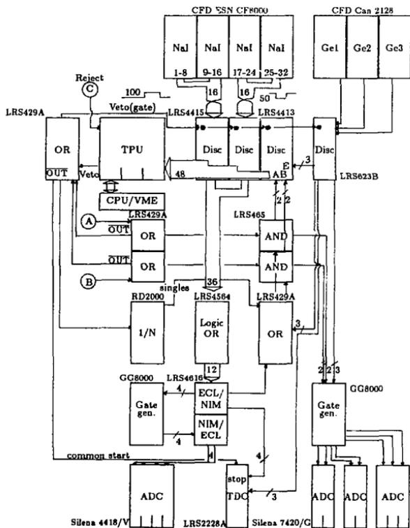
Figure 5.2: The timing set-up for CACTUS. Signals from the particle telescopes 1 - 4 and 5 - 8 are given as inputs at A and B, respectively.
