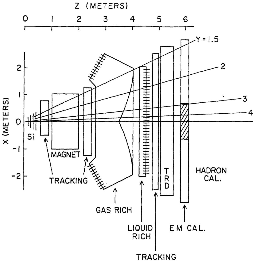
**Fig. 2** Layout of a fixed target experiment. The hash-marks on the Ring Imaging Cerenkov (RICH) counters indicate read-out planes. The shaded portion of the EM calorimeter requires special technology for very intense radiation environments.
