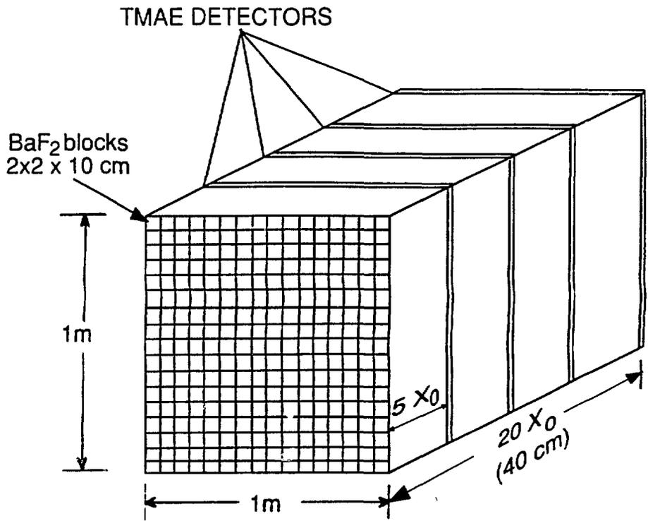
Fig. 10 An electromagnetic shower detector array consisting of 4
