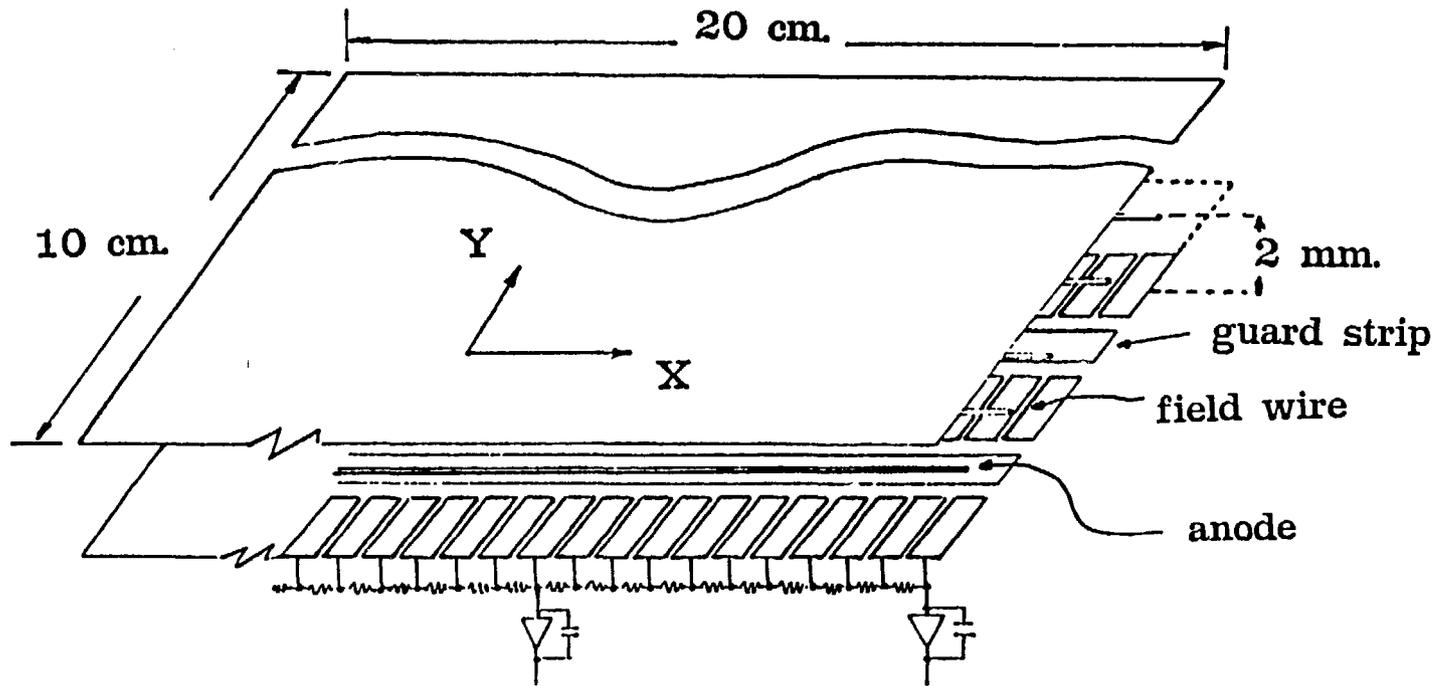
**Fig. 7** Schematic representation of a small pad chamber, with 2 mm cell size and a total of 500 signal channels.
