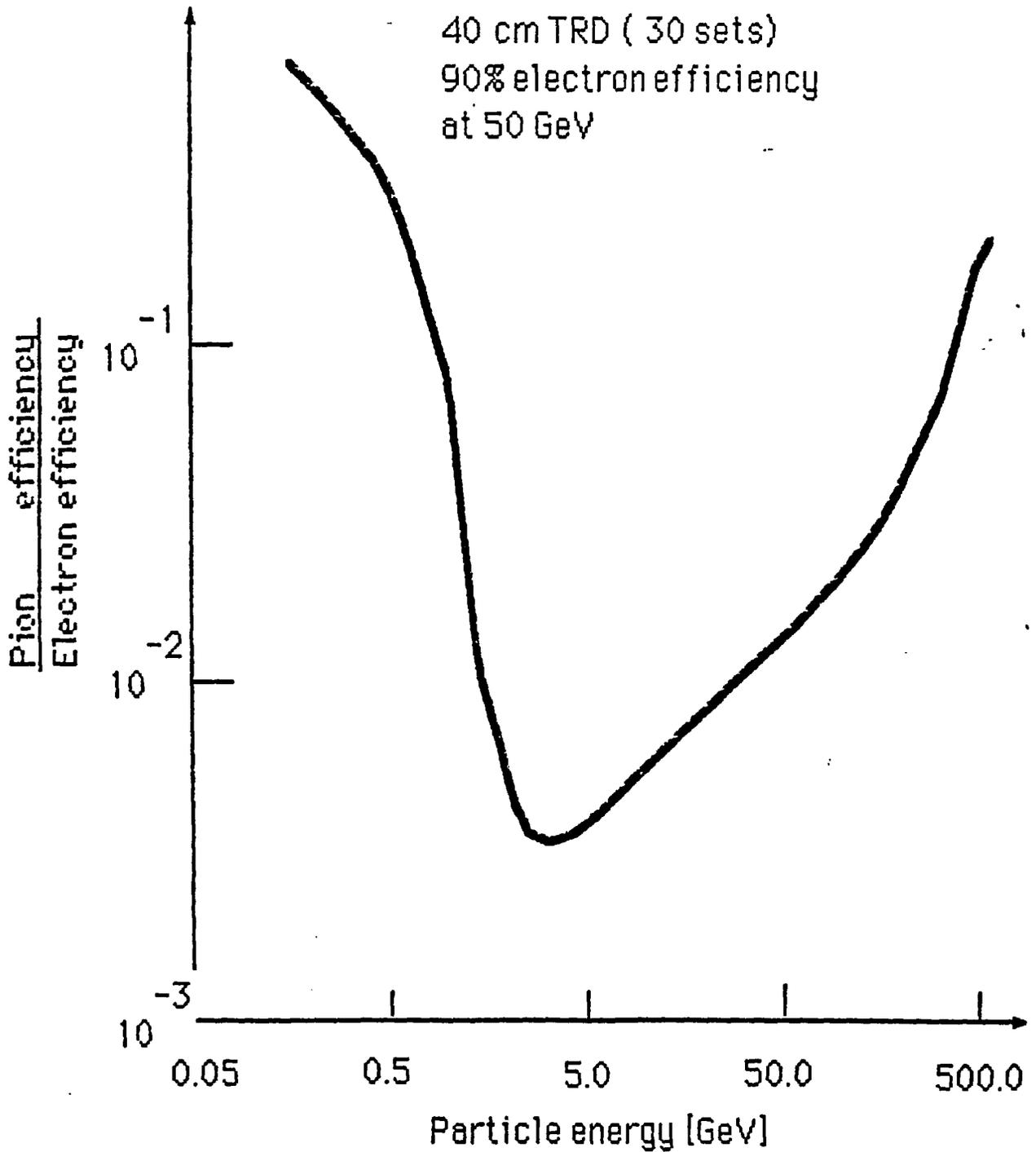
Fig. 6 Hadron rejection power of a 40 cm long TRD made up of modules as shown in Fig. 5 (Ref. 0)
