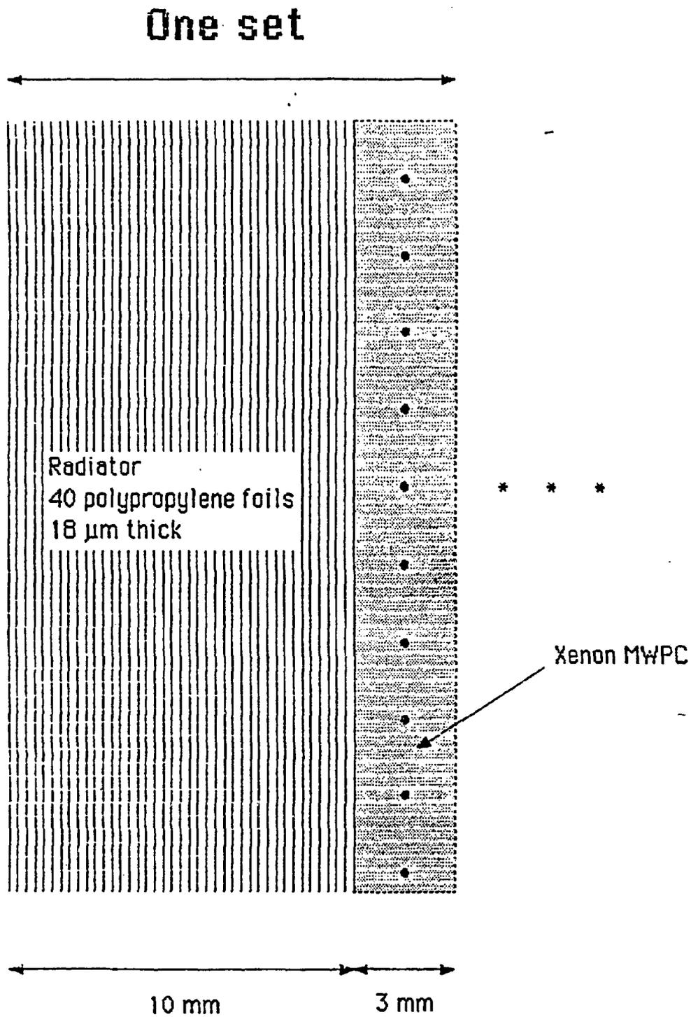
Fig. 5 Schematic layout of a high-granularity cluster-counting TRD (Ref. 9).
