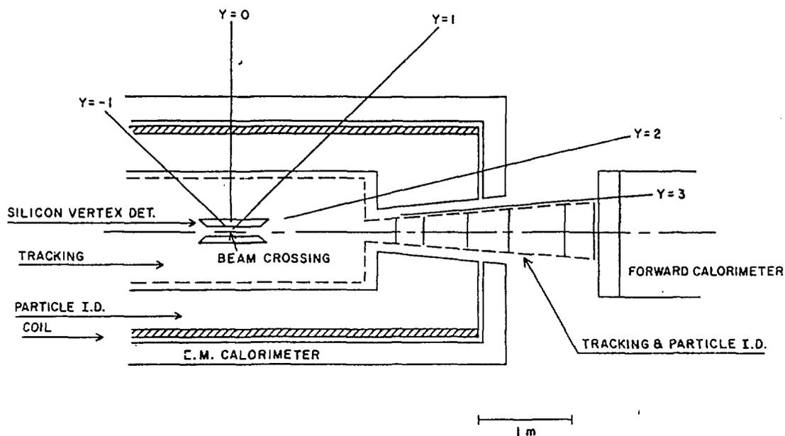
Fig. 1 Detector layout for a B-physics experiment in a collider.
