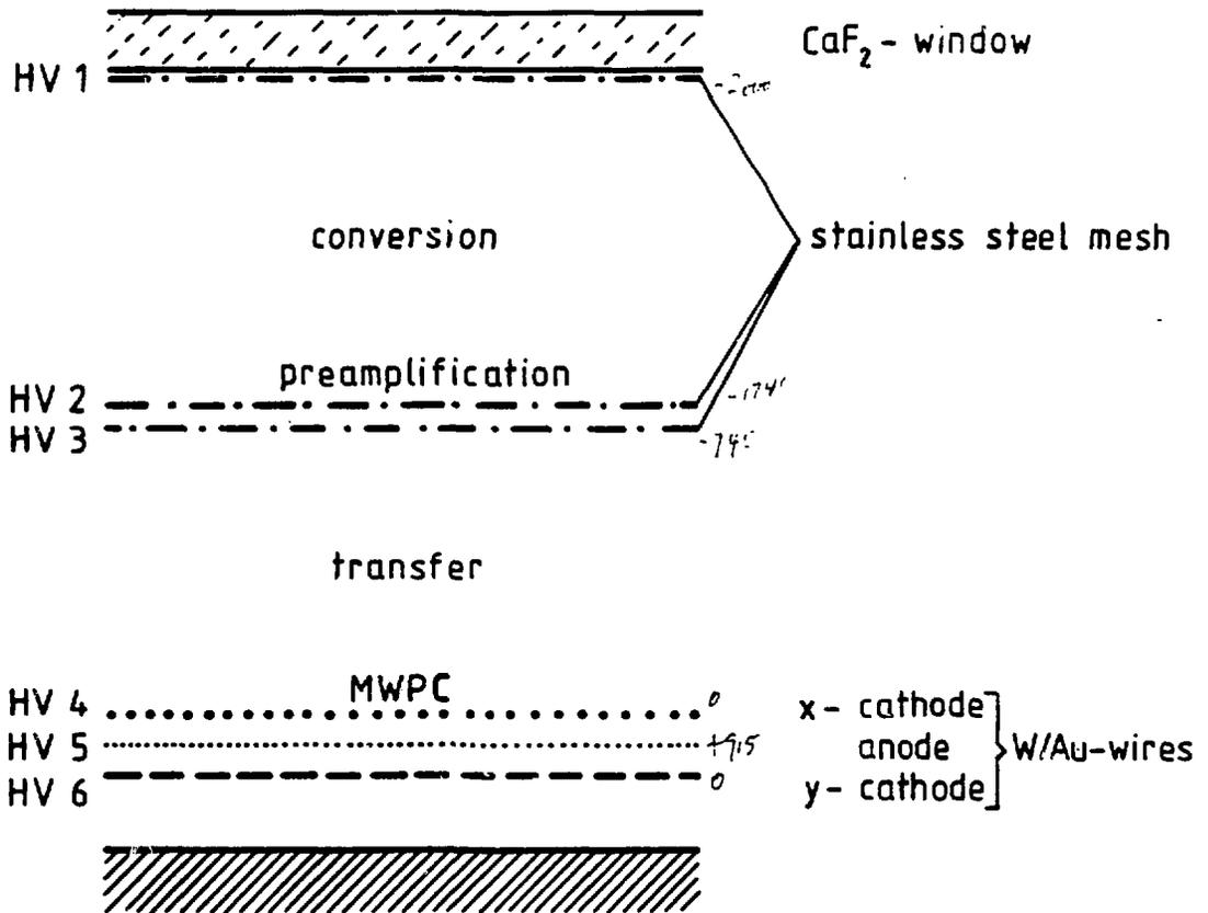
Fig. 9 UV photon conversion and MWPC readout for a Ring Imaging Cerenkov Counter (Ref. 18).
