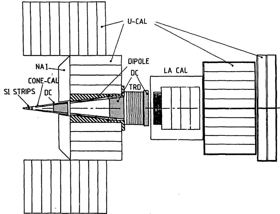
Fig. 3 The HELIOS detector system at the CERN SPS.
