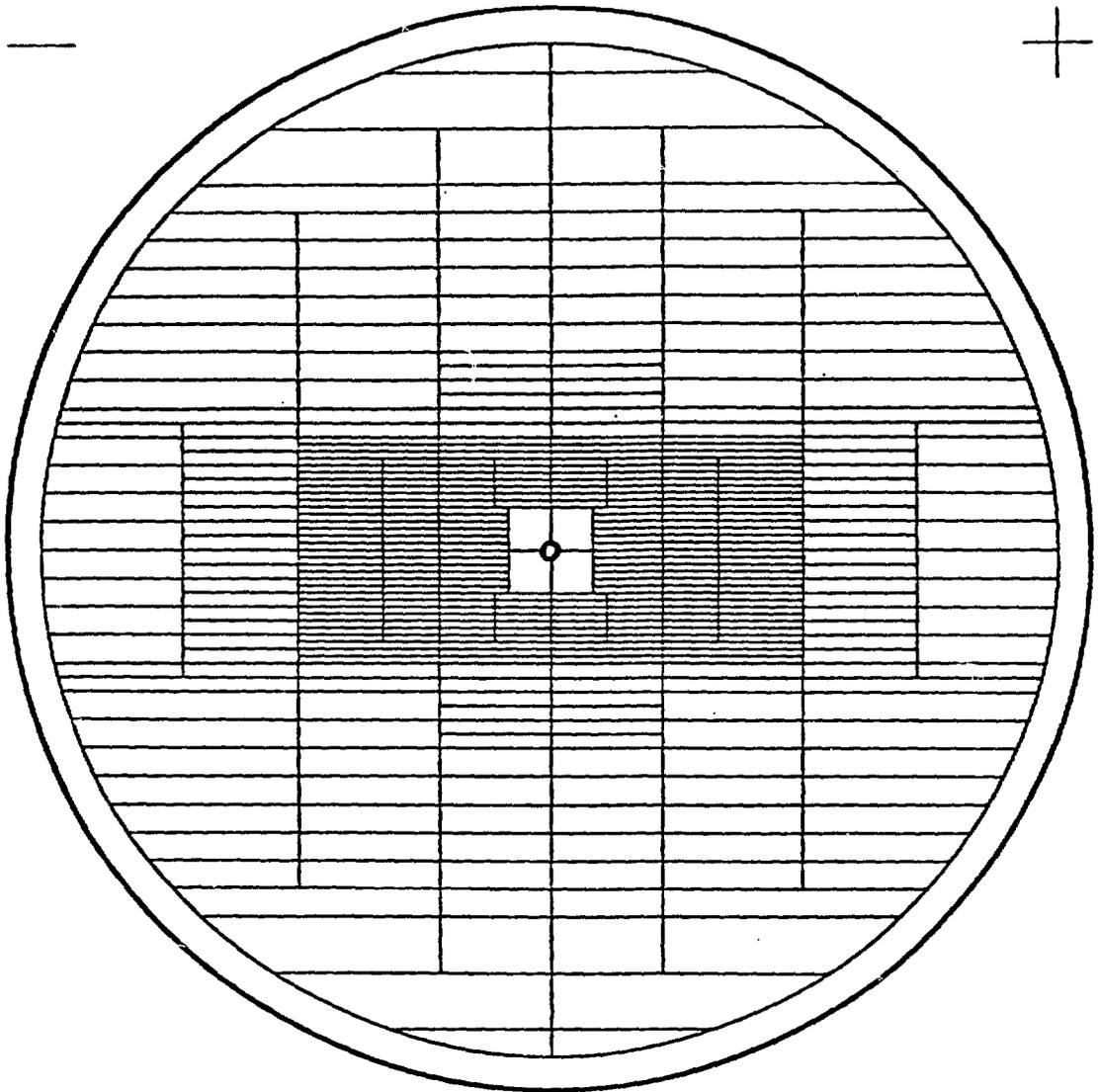
Fig. 4c Segmentation of the HELIOS silicon pad plane.
