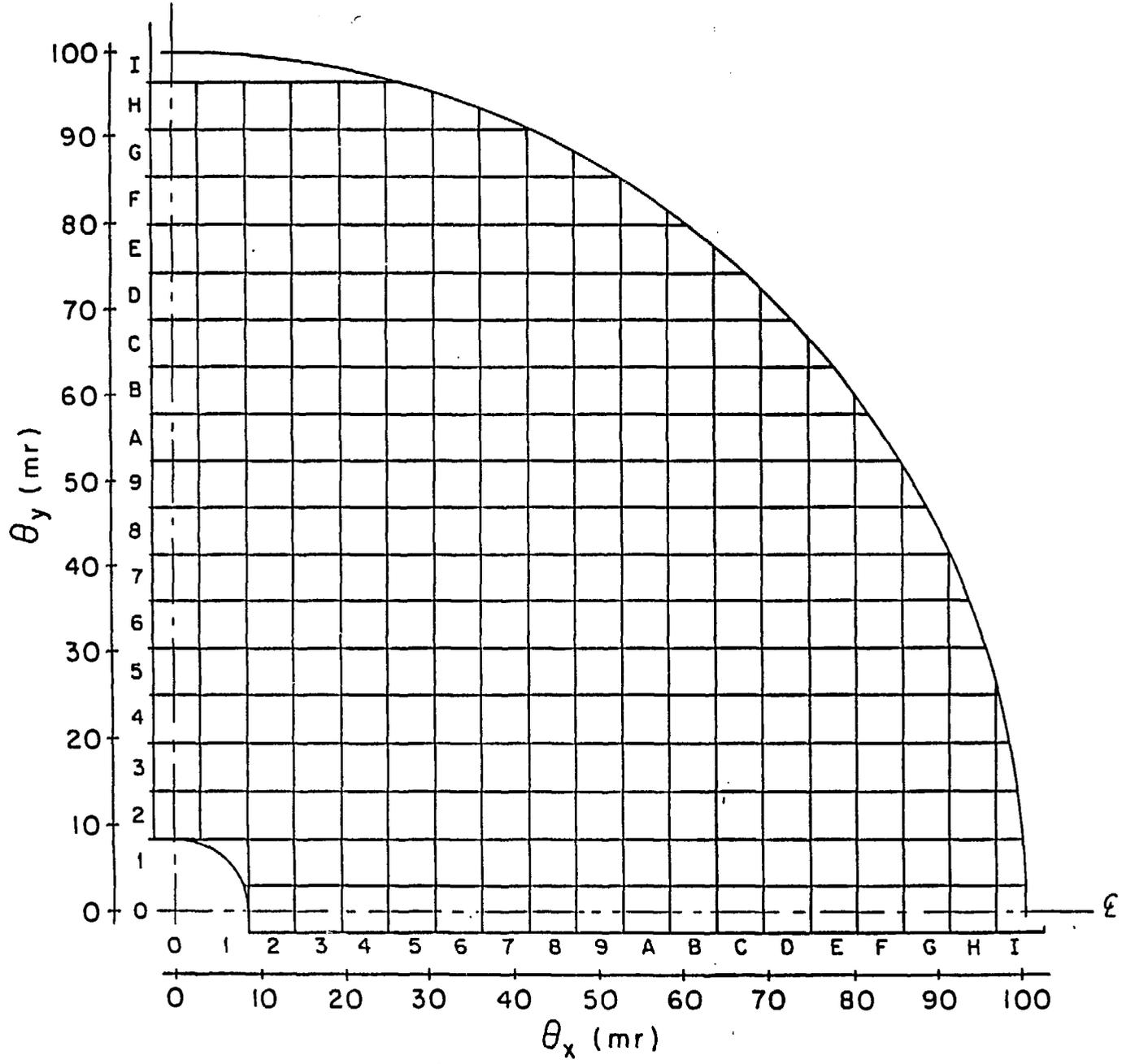
Fig. 4a Segmentation of the electromagnetic portion of the HELIUS uranium/liquid argon calorimeter.
