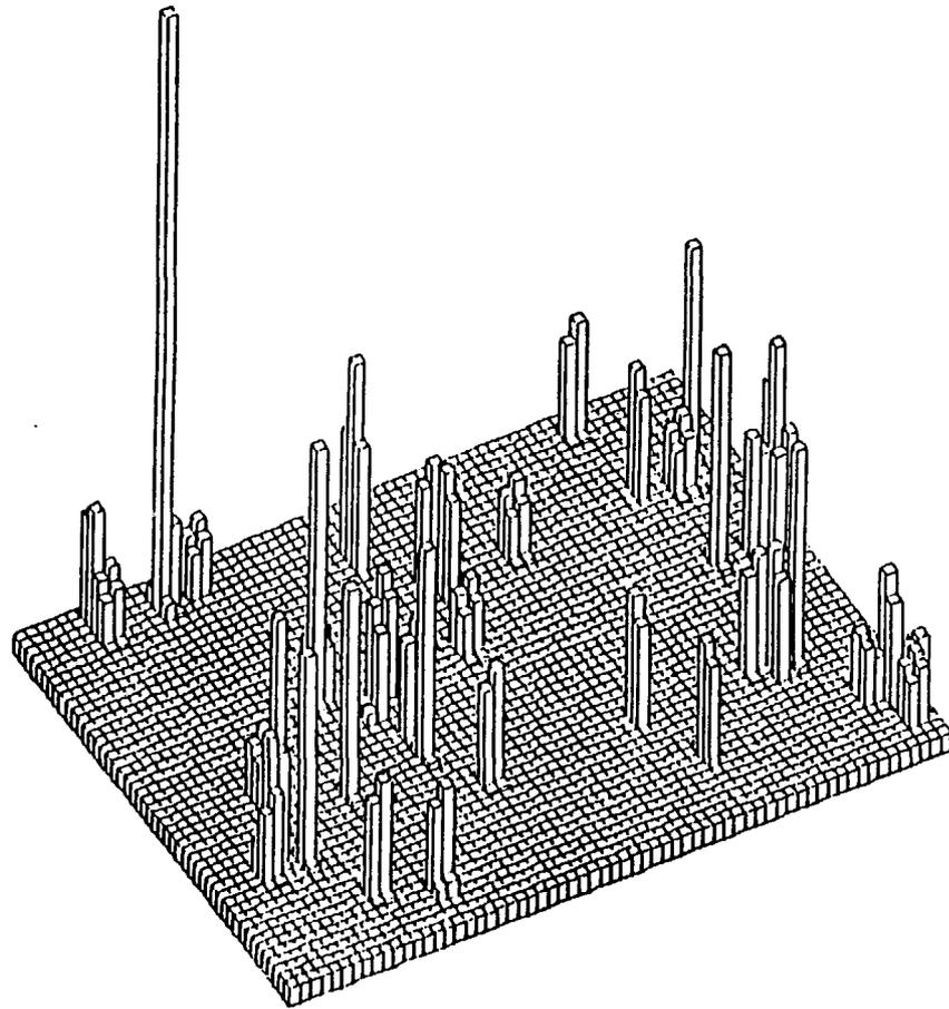
Fig. 8 A Monte Carlo Simulation of 40 minimum ionizing tracks traversing a thin gas chamber with induced charge readout in 3000 pixel-like  $2 \times 2 \text{ mm}^2$  elements for an anode-cathode spacing of 2 mm. The effect of delta rays is included.
