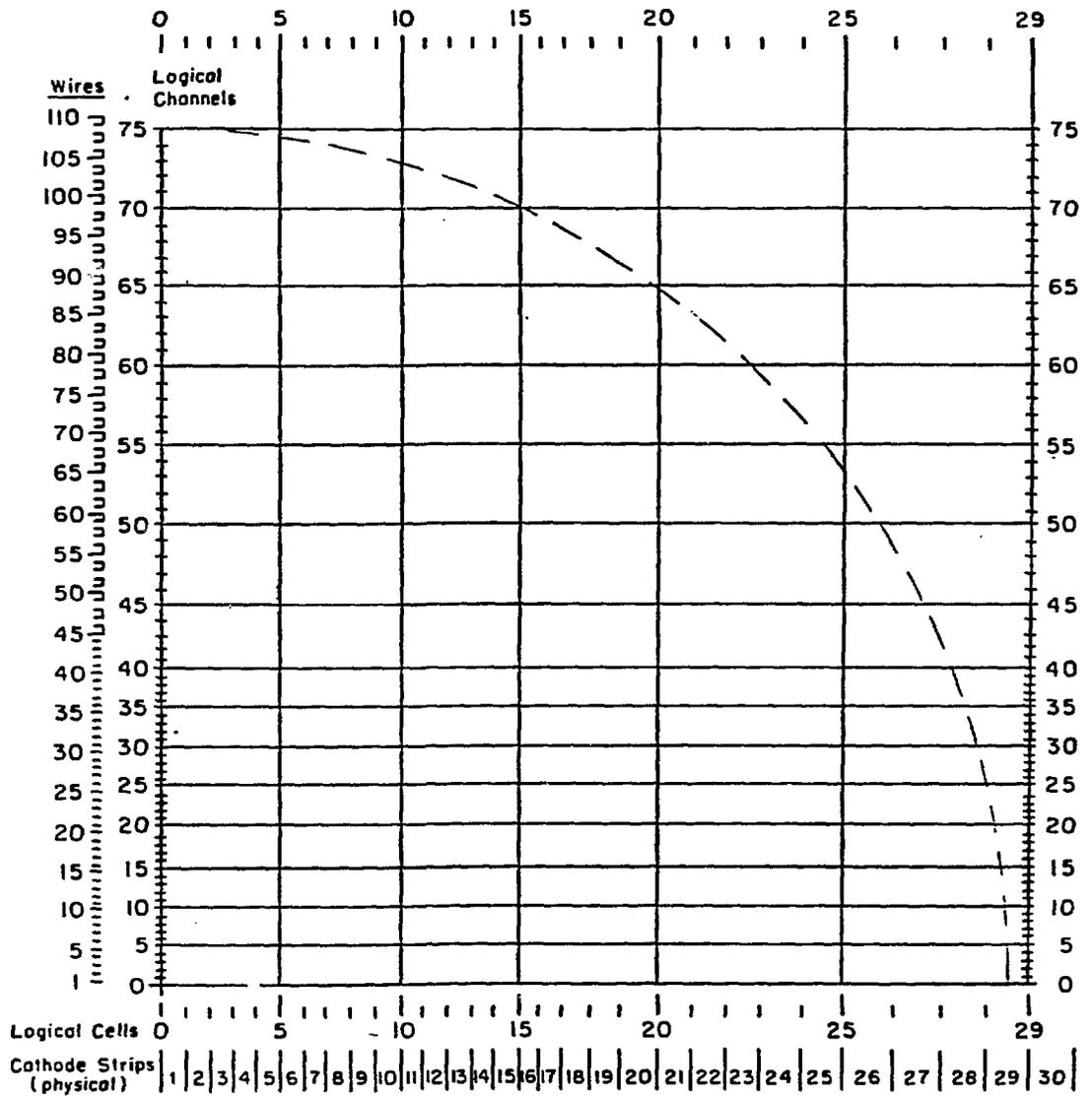
Fig. 4b Segmentation of the HELIOS Transition Radiation Detector readout.
