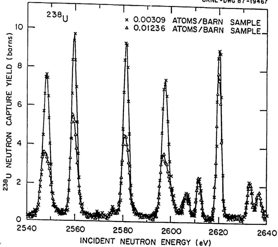
Fig. 13. Capture Yield Data for the 0.00309 atoms/barn and 0.01236 atoms/barn Samples in the Neutron Energy Range from 2540 eV to 2640 eV. The lines shown merely connect the data symbols for each sample for clarity. Note the appearance of substantial sample thickness effects on the larger resonances.
