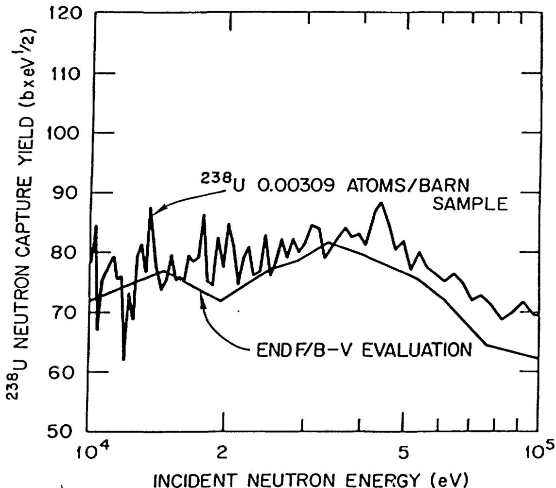
Fig. 20. Comparison of the Intermediate Structure Observed in the Capture Yield Data for the 0.00309 atoms/barn Sample with the Structure Introduced in the  $^{238}\text{U}$  Capture Cross Section by the ENDF/B-V Evaluation (Reference 33) in the Neutron Energy Range from 10 keV to 100 keV. The data have been averaged over 250-channel intervals. Because of the lack of sample thickness corrections in the capture yield data, the present comparison is only intended to be of a qualitative nature.
