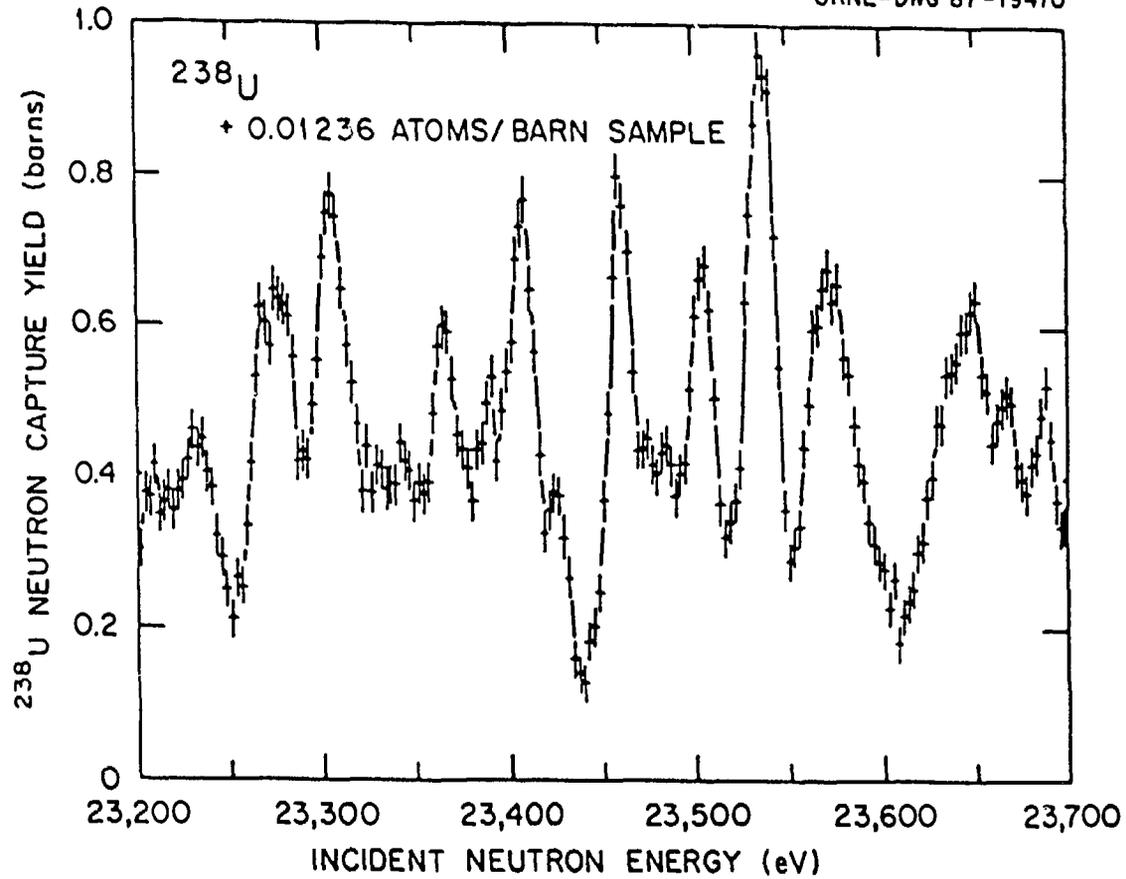
Fig. 16. Capture Yield Data in the Neutron Energy Range from 23.2 keV to 23.7 keV for the 0.01236 atoms/barn Sample. Note the high resolution achieved by the present measurement which is a factor of three better than any previous measurement in this energy region. The vertical bars indicate statistical uncertainties only.
