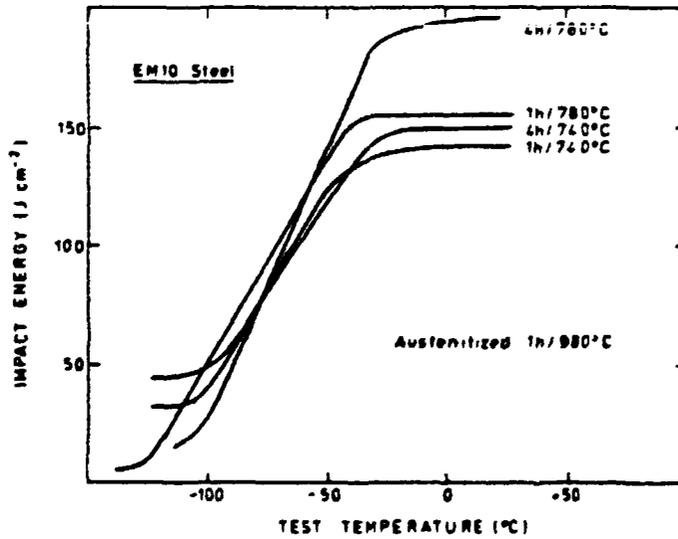
Fig. 4. Effect of tempering on DBTT of EM10 steel.
