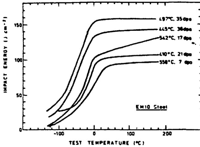
Fig. 9. DBTT data for irradiated EM10 steel.
