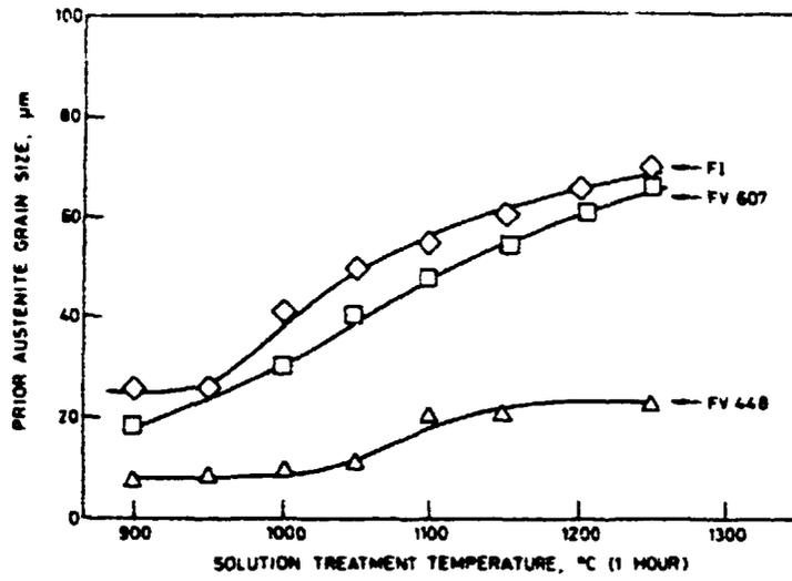
Fig. 3. Prior austenite grain growth characteristics of FI, FV607 and FV448 steels.
