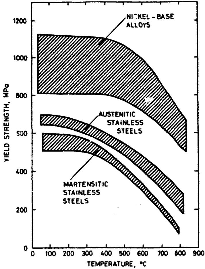
Fig. 1. Schematic of relative yield strengths of martensitic, austenitic and nickel-base alloys.
