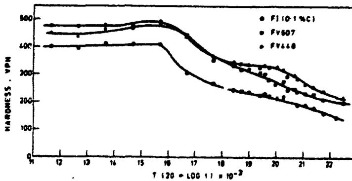
Fig. 2. Tempering characteristics of FI, FV607 and FV448 steels.
