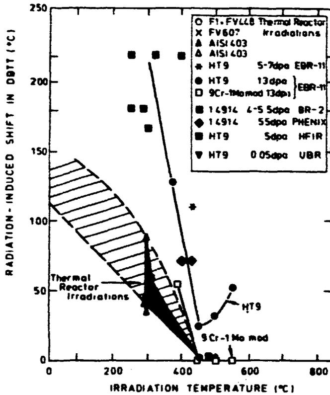
Fig. 11. DBTT shifts as a function of irradiation temperature for a range of 9-12Cr alloys.
