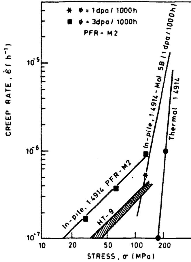
Fig. 15. Thermal and in-reactor creep at 500°C of 1.4914 and HT9 steels.
