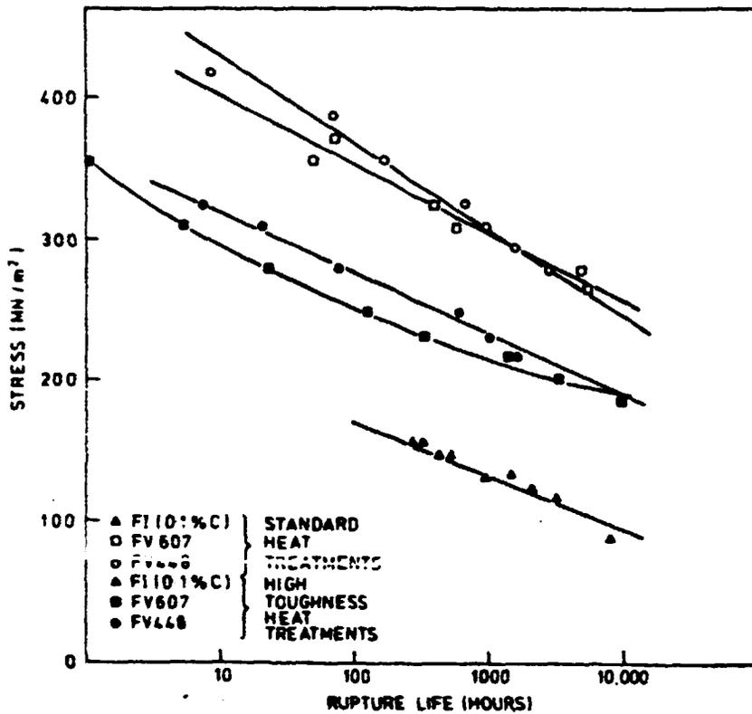
Fig. 5. Stress-rupture data at 550°C for FI, FV607 and FV448 steels as a function of heat treatment.
