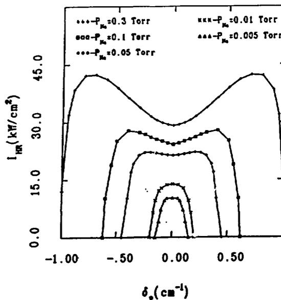
Fig. 4. Theoretical stimulated hyper-Raman output versus detuning from two-photon resonance Na with Na 4d pressures as labeled.
