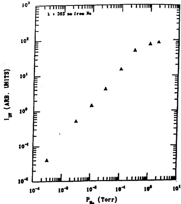
Fig. 2. Parametric four-wave mixing intensity (near 303 nm) versus  $P_{Na}$  for two-photon pumping at  $14\text{ mW/cm}^2$  near Na 4d state.
