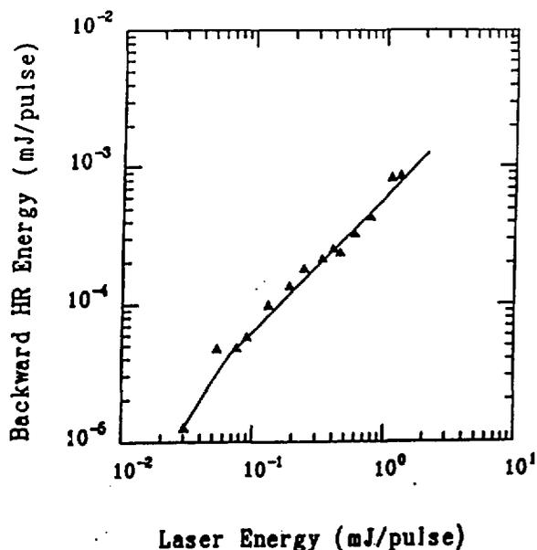
Fig. 3. Backward hyper-Raman output versus laser energy at 0.07 Torr Na.
